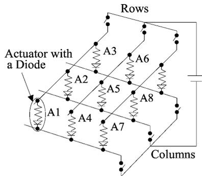
**Fig.5** 3x3 matrix network of SMA actuation (Asada *et al.*, 2000-2002)
