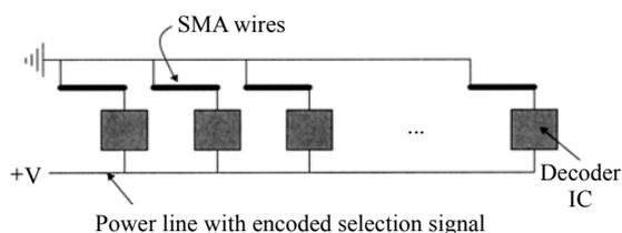
**Fig.10 Control system with decoder for multiple SMA actuators (Sujan and Dubowsky, 2004)**
