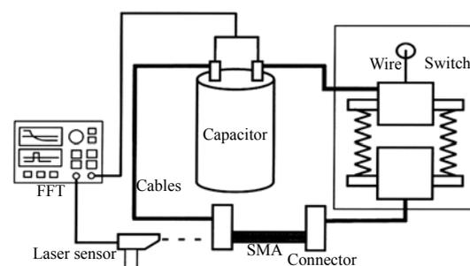
**Fig.2 Electric heating using capacitor (Qiu *et al.*, 2000)**
