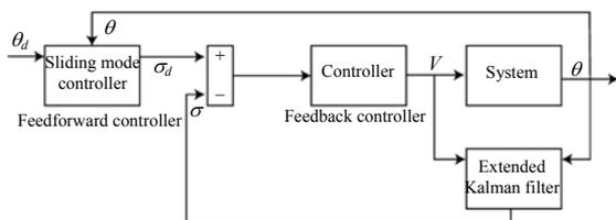
**Fig.7 Feed forward-feed back controller with extended Kalman Filter (Elahinia *et al.*, 2004a)**
