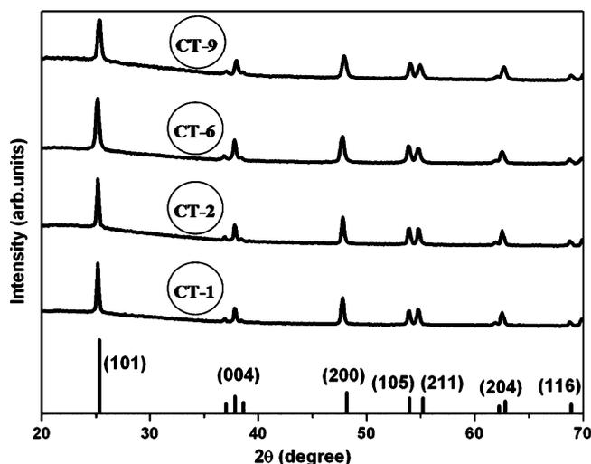
**Figure 4.** XRD profiles of the four different morphologies of C-TiO<sub>2</sub>. For comparison, XRD of bulk anatase TiO<sub>2</sub> is plotted in the bottom (JCPDS 89-4921).
