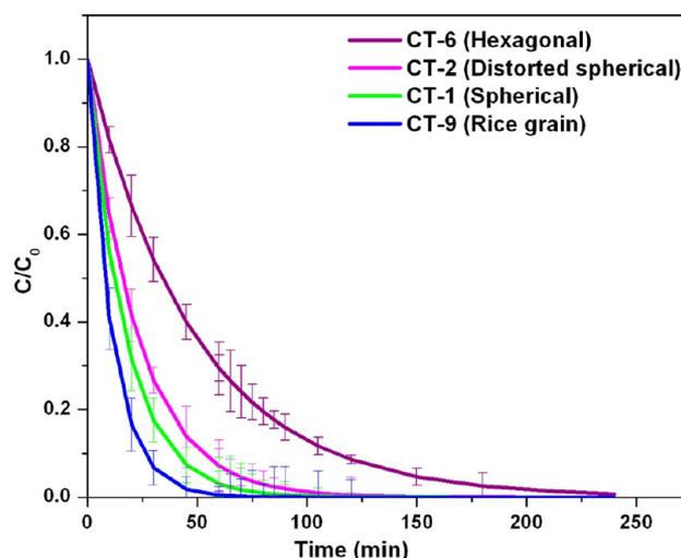
**Figure 7.** Degradation of carbamazepine by different morphologies of C-TiO<sub>2</sub>NCs.
