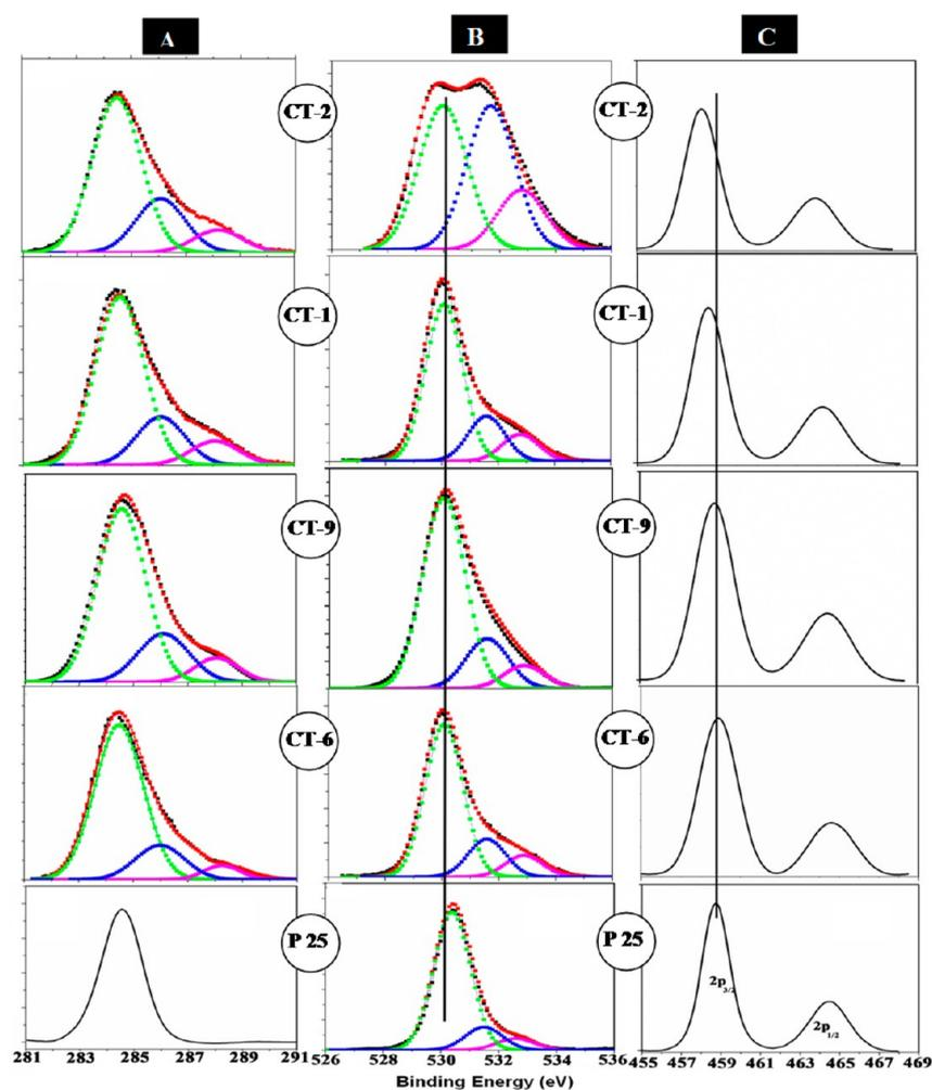
**Figure 6.** XPS of CT-1, CT-2, CT-6, and CT-9 C-TiO<sub>2</sub> samples. For comparison, XPS of bulk TiO<sub>2</sub> (P25 Degussa) is plotted in the bottom. (A) C 1s, (B) O 1s, and (C) Ti 2p. Color scheme: black-experimental curve; red-fitted; green, blue, and pink-deconvoluted species.
