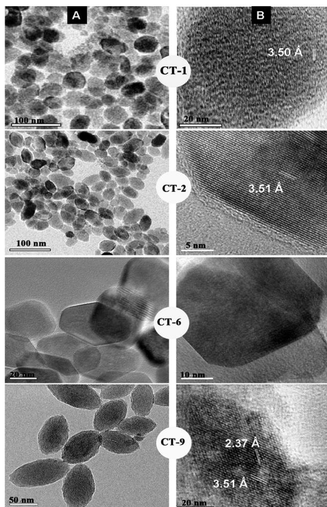
**Figure 3.** TEM images at (A) low and (B) high magnification of spherical (CT-1), distorted spherical (CT-2), hexagonal (CT-6), and rice grain (CT-9) shaped of C-TiO<sub>2</sub> NCs.
