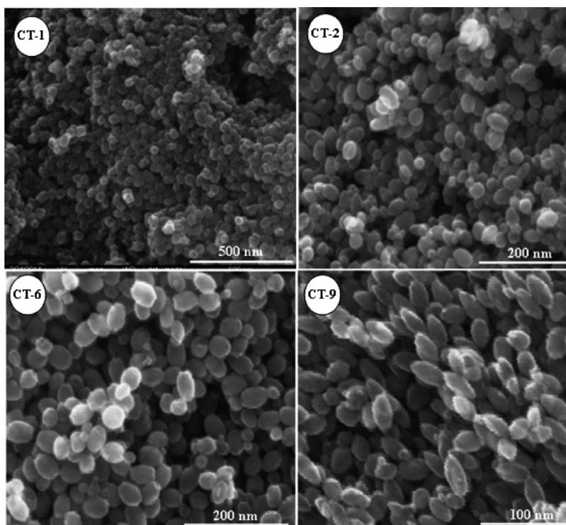
Figure 1. HRSEM images of (CT-1) spherical, (CT-2) distorted spherical, (CT-6) hexagonal, and (CT-9) rice grain shaped C-TiO<sub>2</sub> NCs.
