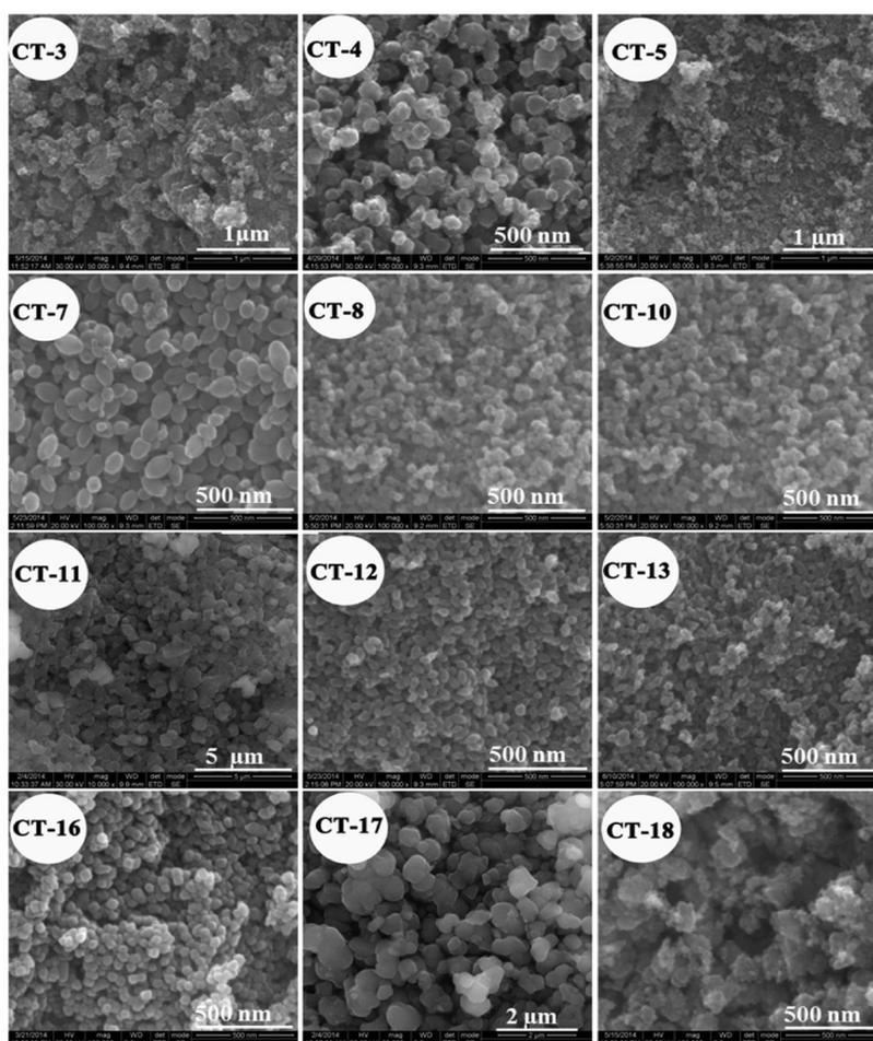
Figure 2. HRSEM images of C-TiO<sub>2</sub> samples prepared using different reaction conditions by microwave digestion technique.
