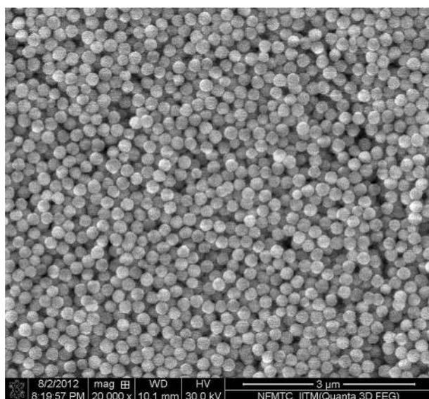
FIG. 1. FESEM image shows the randomly arranged ZnS sub-micron spheres coated over microglass slide.
