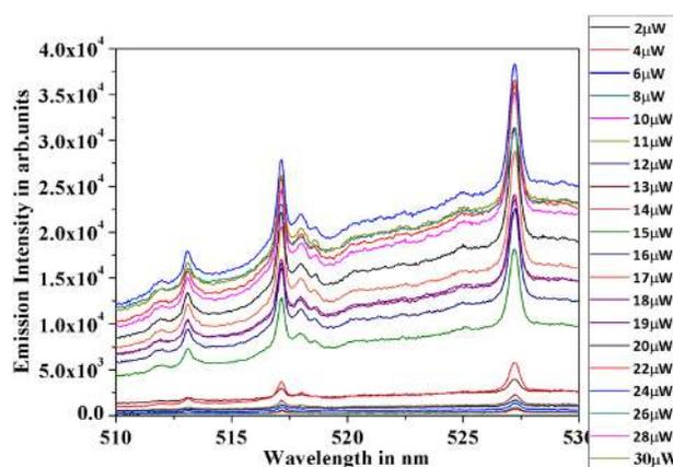
FIG. 4. Emission spectra of ZnS- $\beta$ -carotene composite random media with Raman lasing at 513 nm, 517 nm, and 527 nm.
