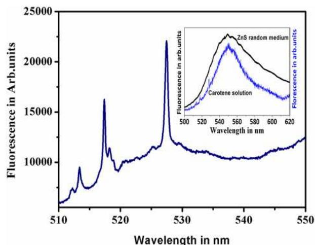
FIG. 3. Emission spectra of ZnS- $\beta$ -carotene random media and the individual emission spectra of ZnS random media and  $\beta$ -carotene molecule.
