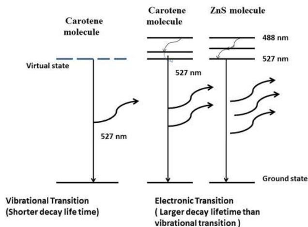
FIG. 6. Energy level diagram indicating the possible vibrational and electronic transitions responsible for random lasing Raman in ZnS- $\beta$ -carotene composite random media.
