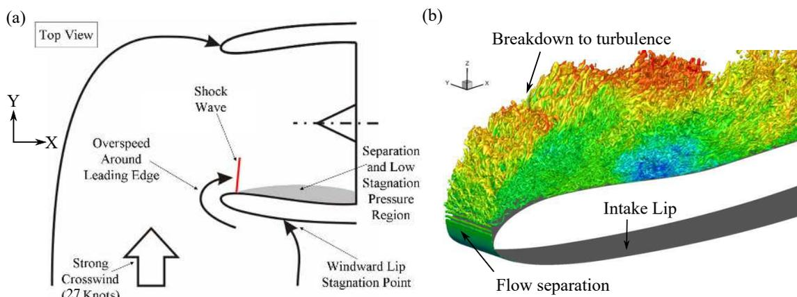
**Figure 1.** (a) Flow over an intake under crosswind [11]; (b) low-speed separation on intake lip (Vadlamani and Tucker [5]).
