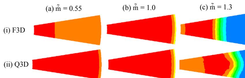
**Figure 12.** Comparison of stagnation pressure contours in a 20° sector at the fan face.
