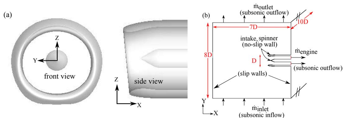
**Figure 2.** (a) Drooped intake geometry; (b) boundary conditions for full 3D simulations.
