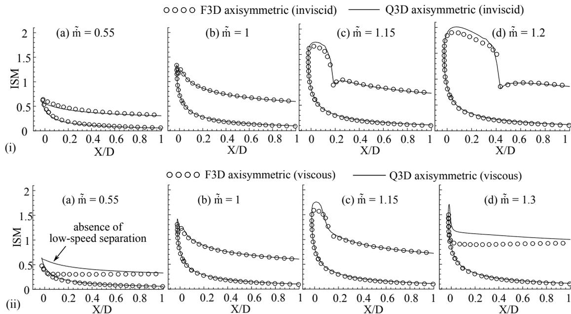
**Figure 11.** Variation of ISM with axial distance for F3D axisymmetric and Q3D cases with (i) inviscid BC and (ii) viscous no-slip BC on the intake lip.
