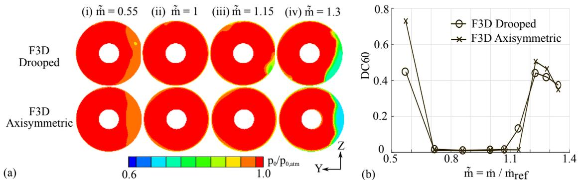
**Figure 6.** Drooped and axisymmetric cases: comparison of (a)  $P_0$  and (b) DC60 at fan face.
