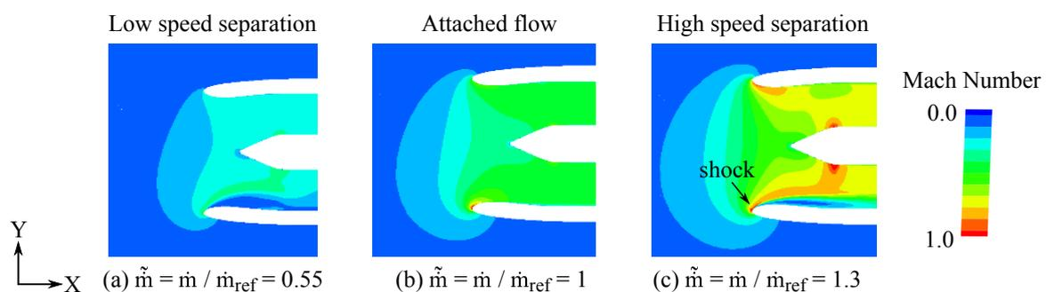
Figure 3. Mach number contours on  $Z = 0$  plane for increasing engine mass flow rate.
