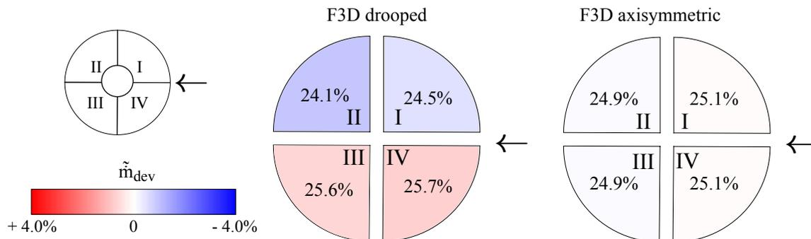
**Figure 7.** Distribution of mass flow at fan face quadrants for F3D drooped and axisymmetric viscous simulations, when  $\tilde{m} = 1$  (pie colours represent  $\tilde{m}_{dev}$ ).
