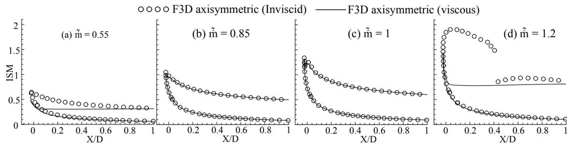
Figure 8. Axial variation of ISM for F3D axisymmetric viscous and inviscid simulations.
