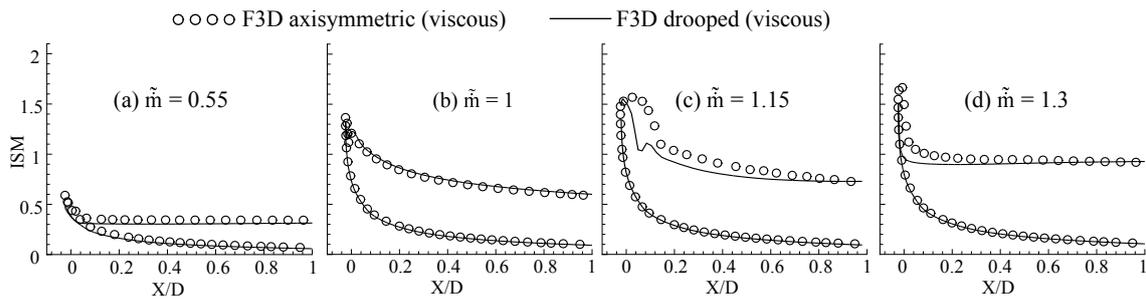
**Figure 5.** Axial variation of isentropic Mach number (ISM) for free 3D (F3D) drooped and axisymmetric viscous simulations.
