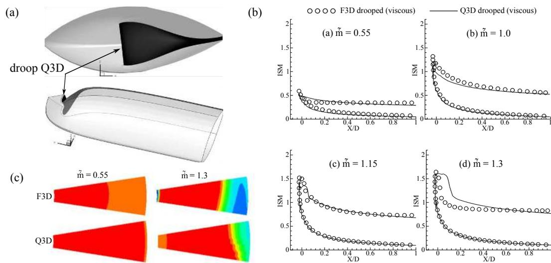
**Figure A1.** (a) Q3D drooped duct (b) ISM and (c)  $P_0$  contours for F3D, Q3D drooped cases.
