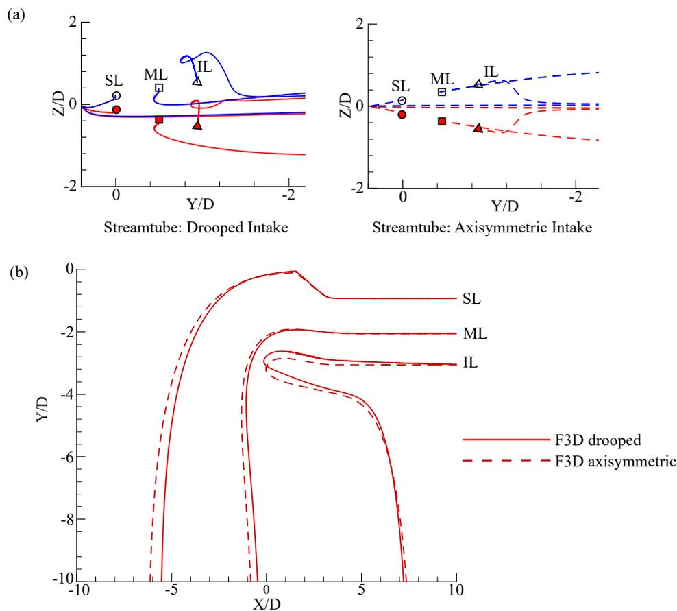
**Figure 10.** F3D captured streamtubes for  $\tilde{m} = 1$  obtained from F3D drooped and axisymmetric simulations (a) in the Y – Z plane; (b) in the X – Y plane.
