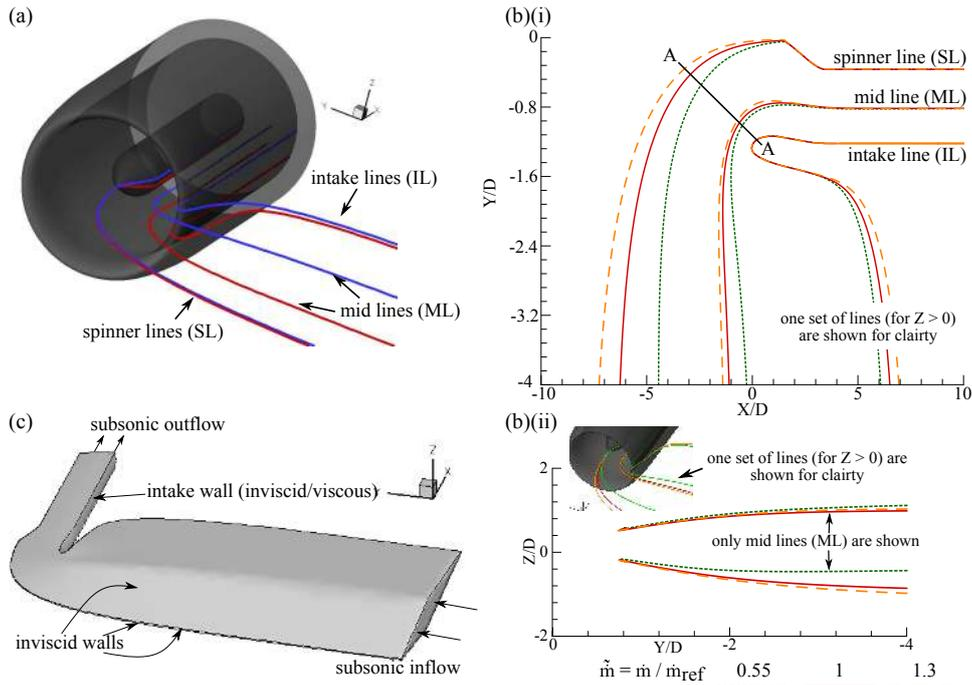
**Figure 9.** (a) Captured streamtube for  $\tilde{m} = 1$ , for F3D axisymmetric intake; (b) captured streamtube at different mass flow rates; (c) 3D view of axisymmetric quasi-3D (Q3D) duct with corresponding Boundary Conditions (BCs).
