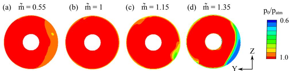
**Figure 4.**  $P_0$  contours at fan-face: (a) low-speed separation; (b) attached flow; (c,d) high speed separation.
