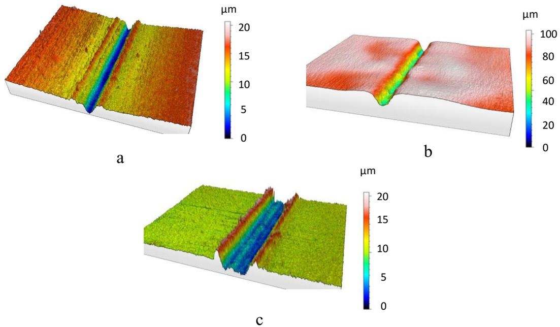
**Figure 5:** 3D images of the micro channels produced using 532 nm laser wavelength using a) 35 mJ energy using a Gaussian beam on copper thin film b) 7 mJ of energy using a Gaussian beam on an aluminum thin film c) 35 mJ of energy using a flat-top profile on a copper thin film. Measurements were performed using Marsurf CWM 100.
