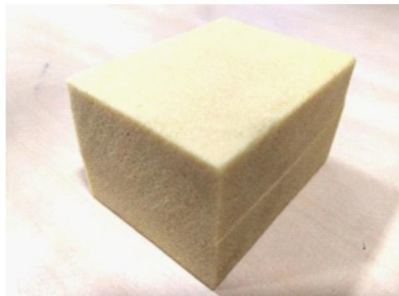
Fig. 1. Rigid polyurethane foam with 300 kg/m<sup>3</sup> density.
