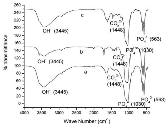
Fig. 2. FT-IR spectra of TH980.5L (a) TH981.5L (b) and TH901.0L (c) samples.
