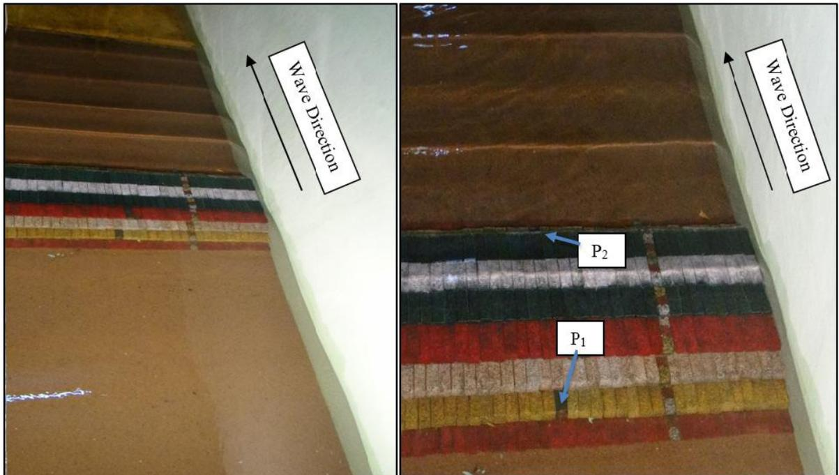
Fig. 2 (a) Wave Transformation past the reef (b) Location of Pressure gauges on GBAR
