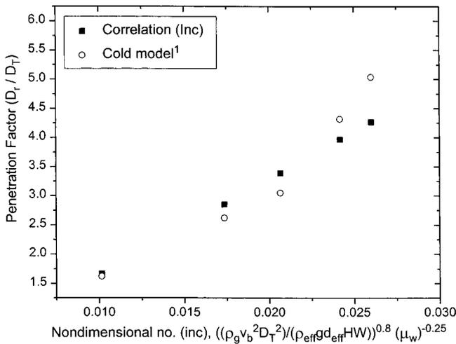
Fig. 6. Comparison of penetration factors obtained from correlation and published<sup>1)</sup> data of 0.725 mm ballotini glass.
