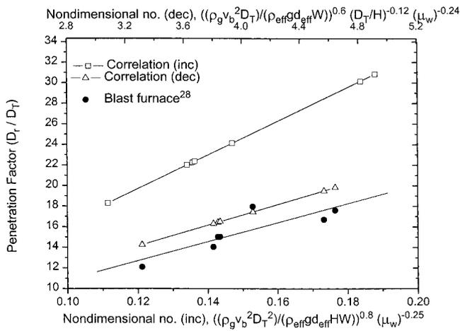
Fig. 10. Comparison of correlations with published blast furnace data of Nishi *et al.*<sup>28)</sup>
