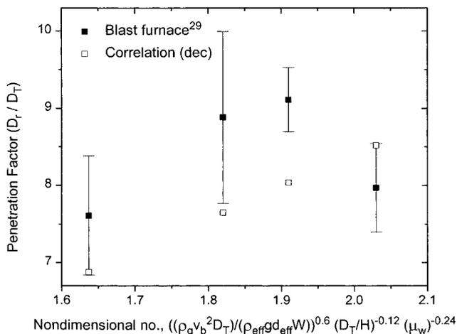
Fig. 11. Comparison of penetration factors obtained from correlation with published blast furnace data<sup>29)</sup> of various furnaces.
