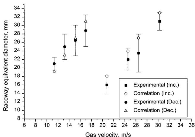
Fig. 4. Comparison of raceway diameter between experimental and correlations in both increasing and decreasing velocity.
