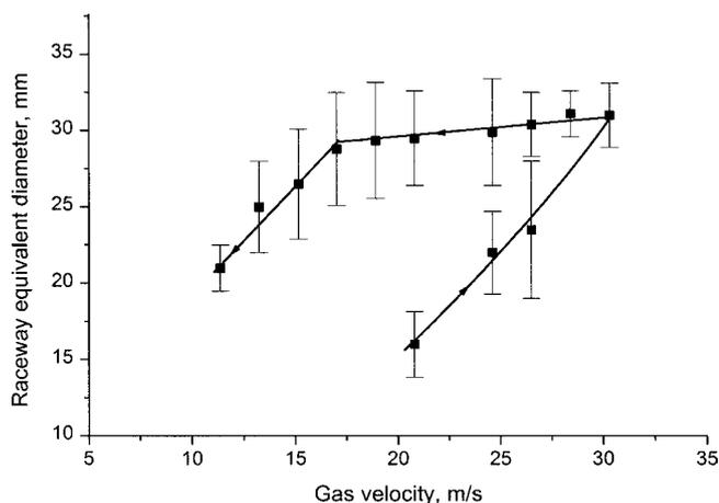
Fig. 3. Experimental raceway hysteresis for plastic beads of 2.1 mm size.
