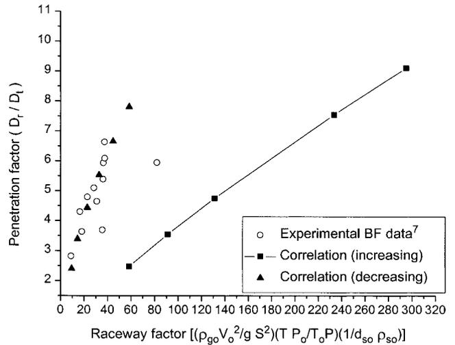
Fig. 7. Comparison of experimental blast furnace<sup>7)</sup> and cold model data for both increasing and decreasing velocity conditions.
