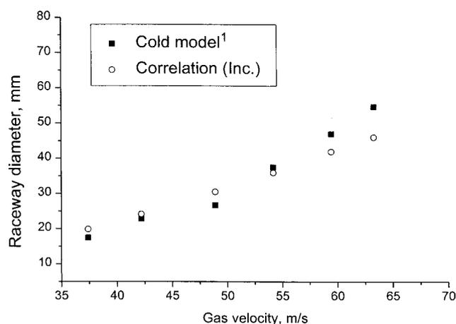
Fig. 5. Comparison of correlation raceway diameter with published<sup>1)</sup> data of 3 mm polystyrene.
