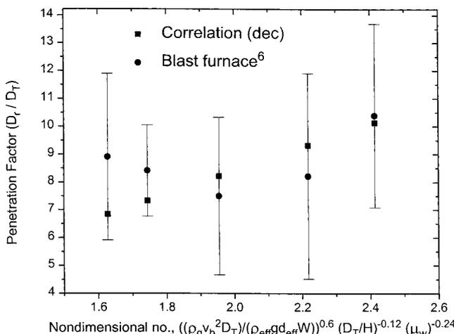
**Fig. 9.** Comparison of penetration factors obtained from correlation with published blast furnace data<sup>6)</sup> of various furnaces.
