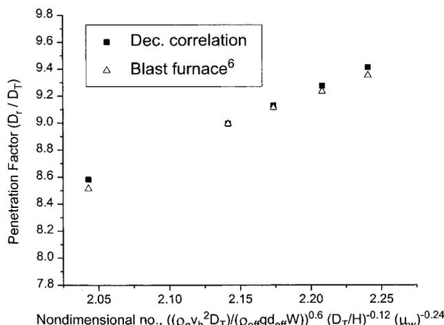
**Fig. 8.** Comparison of penetration factors obtained from decreasing correlation with published blast furnace data<sup>6)</sup> for one furnace.
