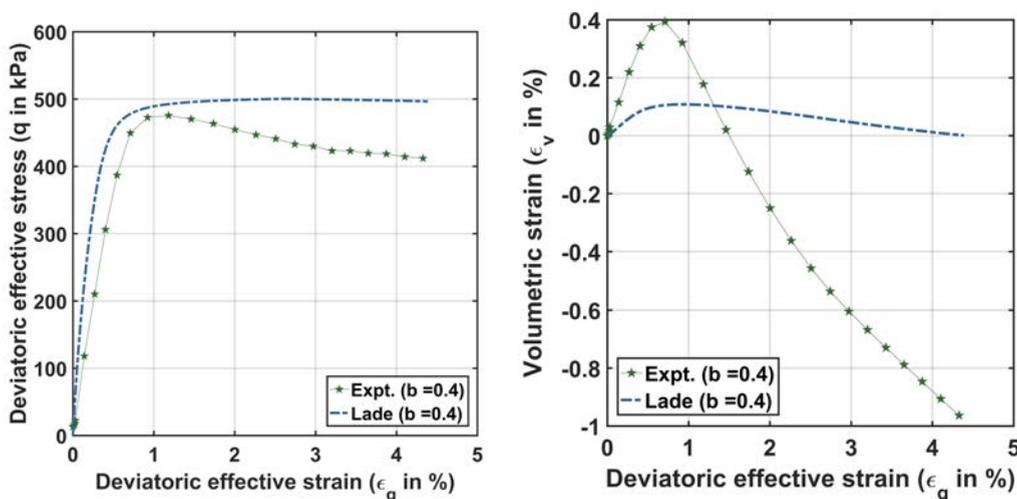
Fig. 3: a: Comparison of predicted and experimentally obtained response of stress strain behaviour at  $b = 0.4$  and mean effective stress ( $p'$ ) of 300 kPa b: Comparison of predicted and experimentally obtained response of volumetric behaviour at  $b = 0.4$  and mean effective stress ( $p'$ ) of 300 kPa
