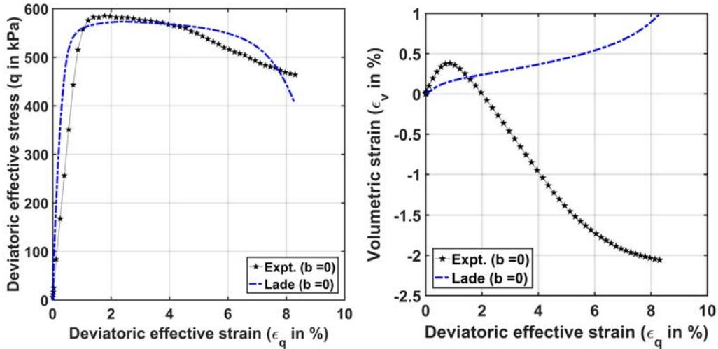
Fig. 1: a: Comparison of predicted and experimentally obtained response of stress strain behaviour at  $b = 0$  and mean effective stress ( $p'$ ) of 300 kPa b: Comparison of predicted and experimentally obtained response of volumetric behaviour at  $b = 0$  and mean effective stress ( $p'$ ) of 300 kPa
