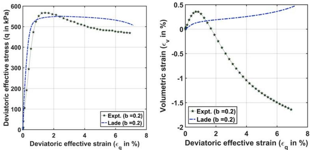
Fig. 2: a: Comparison of predicted and experimentally obtained response of stress strain behaviour at  $b = 0.2$  and mean effective stress ( $p'$ ) of 300 kPa b: Comparison of predicted and experimentally obtained response of volumetric behaviour at  $b = 0.2$  and mean effective stress ( $p'$ ) of 300 kPa
