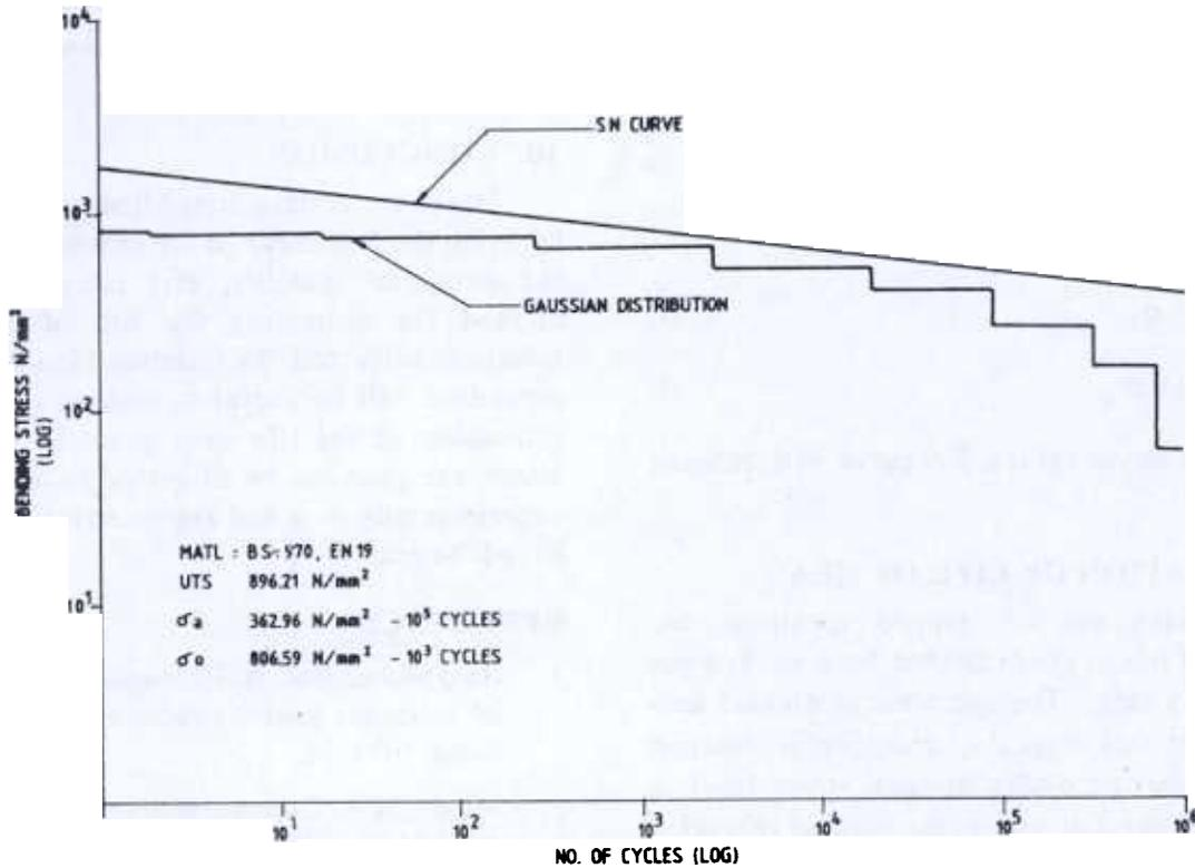
Figure 7. *S-N* curve with stepped Gaussian distribution
