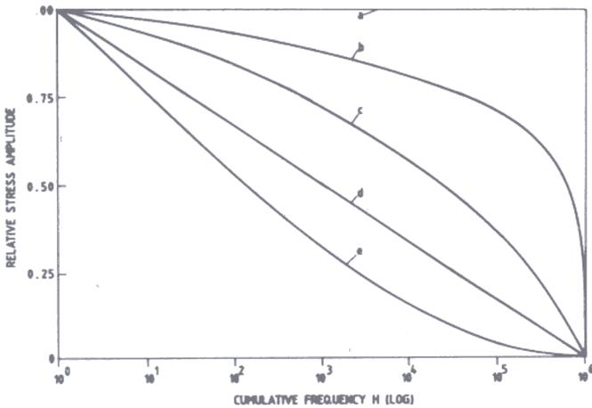
Figure 3. Typical amplitude distributions plotted on relative scale.
