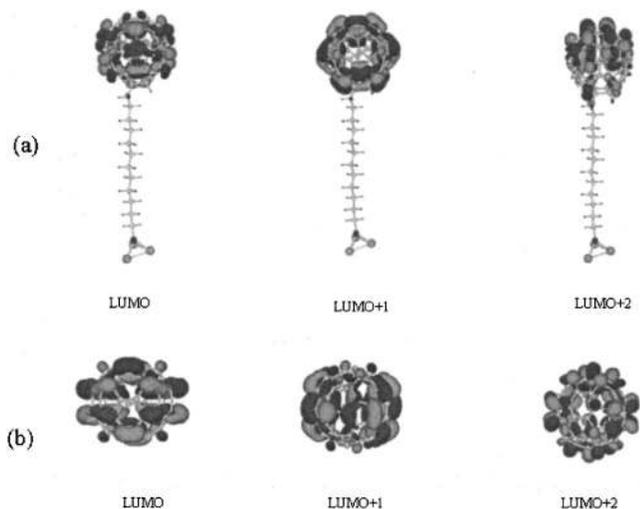
FIG. 7. Typical lowest unoccupied molecular orbitals of (a) C<sub>60</sub>-functionalized 11-AUT, and (b) solid C<sub>60</sub>, calculated from DFT with linear combination of atomic orbitals (LCAO) approach.
