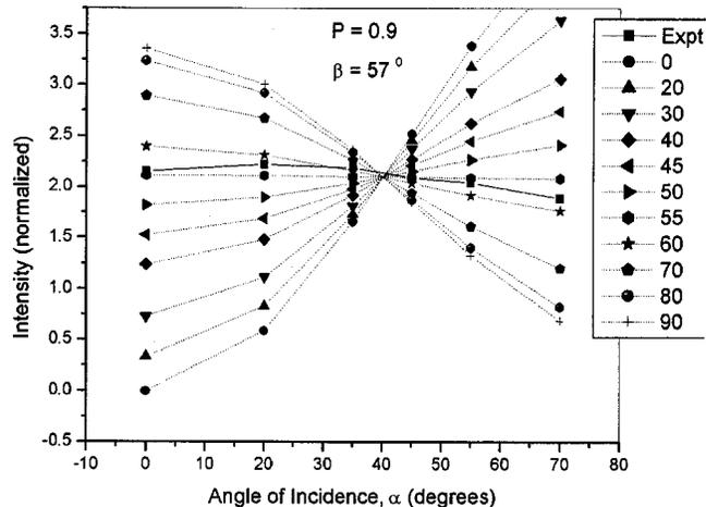
FIG. 3. Graphical representation of normalized NEXAFS intensities of  $\text{C}_{60}$ -functionalized 11-AUT SAM as a function of angle of incidence of photons, according to Eq. (3). The filled squares connected with a solid line are experimental points.
