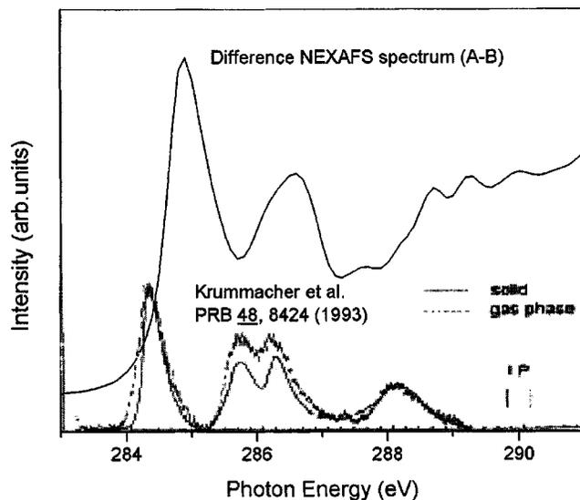
FIG. 5. A comparison between the C 1s near-edge absorption spectrum of (A-B) in Fig. 4 with that of solid and gas phase spectra of C<sub>60</sub> (*vide* Ref. 10). The vertical bars at 290.1 and 289.75 eV indicate C 1s ionization potentials relative to vacuum level for the respective phases.
