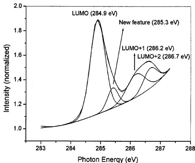
FIG. 6. Gaussian peak fitting of the lower-energy region of the NEXAFS spectrum of C<sub>60</sub>-functionalized 11-AUT illustrating the new (C<sub>60</sub>)<sub>n</sub>  $\pi^*$  feature.
