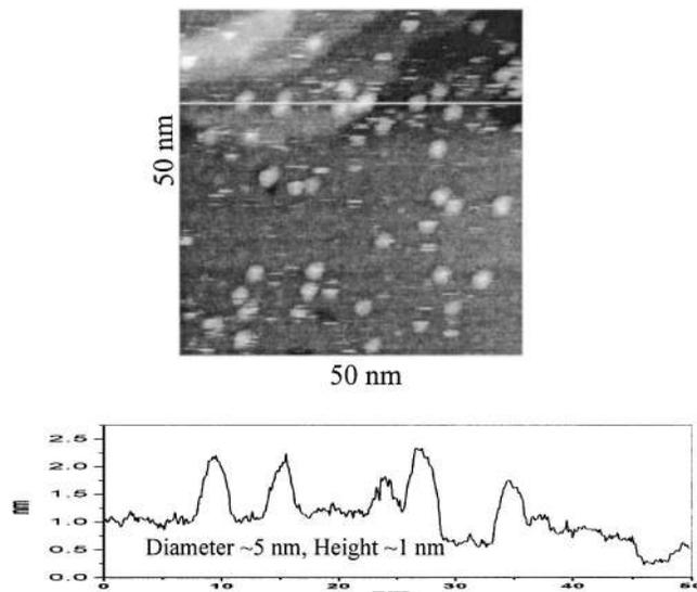
FIG. 8. A 50×50 nm STM image of C<sub>60</sub>-functionalized 11-AUT SAM on Au(111) surface. Image taken at 0.08 nA/400 mV at 1.02 Hz / 1.5 nm.
