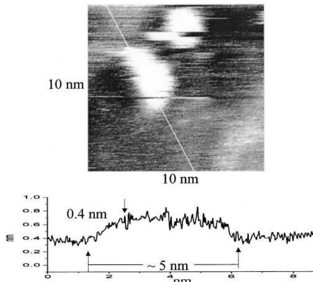
FIG. 9. STM images of 10×10 nm of C<sub>60</sub>-functionalized 11-AUT SAM on Au(111) surface. Image taken at 0.10 nA/500 mV at 5.79 Hz/0.6 nm.
