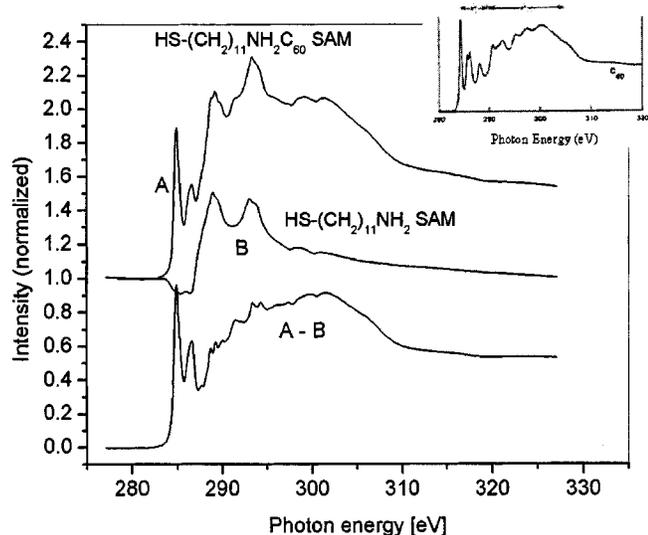
FIG. 4. Comparative NEXAFS spectra shown for 11-AUT SAM on Au(111)→B and the corresponding C<sub>60</sub>-functionalized 11-AUT on Au(111)→A. The difference spectrum (A-B) resembles the NEXAFS spectrum of solid C<sub>60</sub>, shown in the inset, *vide* Ref. 9.
