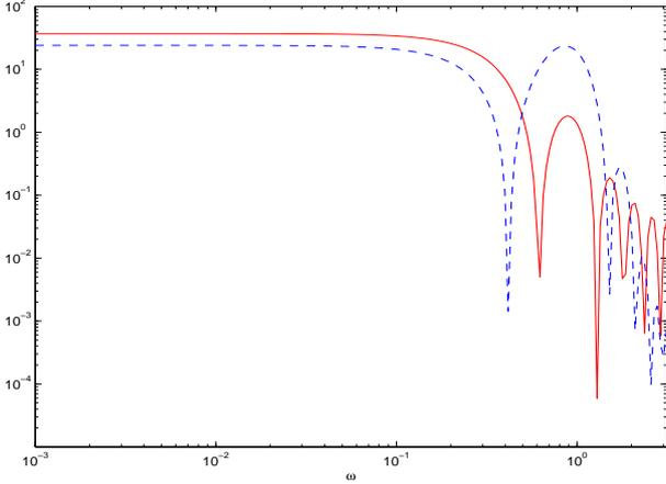
Fig. 3. Flexible spectrum  $\Phi_{r,opt}(\omega)$  without move size constraint (blue dashed) and flexible spectrum  $\Phi_{r,opt,move}(\omega)$  with move size constraints (red solid)
