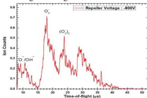
**Figure 1.** TOF spectra for the precursor, oxygen, is presented. In this case, we have used pulsed supersonic discharge ion source (solenoid valve). Supersonic expansion through 150μm nozzle has yielded cluster anion.
