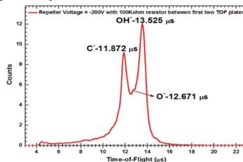
**Figure 2.** TOF spectra with air as the discharge medium. In this case, we have used cold-cathode plasma source. Unlike the supersonic source, this source does not yield cluster anions.
