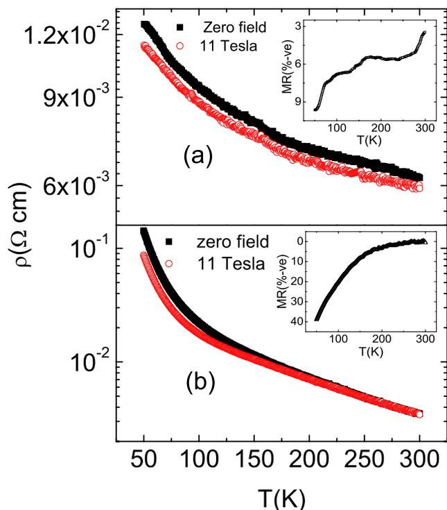
FIG. 4. (Color online) Temperature dependence of resistivity for (a) S1 and (b) S2 in  $H=0$  T and  $H=11$  T. The insets in both the figures display the calculated MR as a function of temperature.
