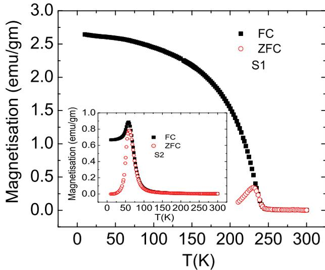
FIG. 1. (Color online) Temperature dependence of FC and ZFC dc magnetizations for S1. The inset shows the same for S2.
