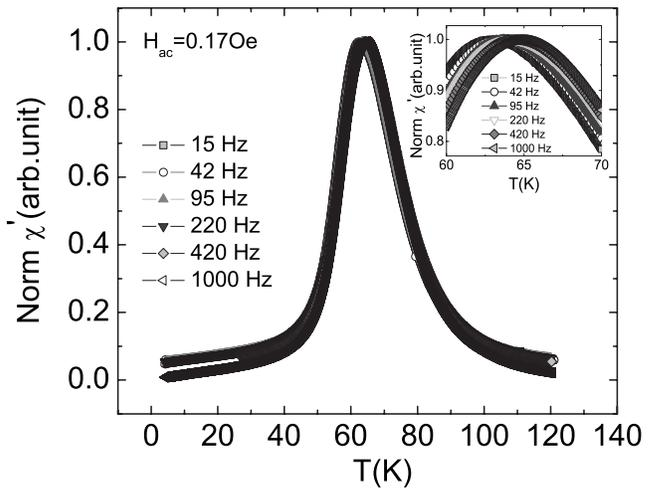
FIG. 2. Temperature dependence of normalized (norm) in-phase component  $\chi'(T)$  of ac susceptibility for S2 in an ac field of  $H_{ac}=0.17$  Oe with frequencies of 15, 42, 95, 220, 420, and 1000 Hz, respectively. The inset shows a close up view of frequency dependent peak shifts.
