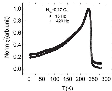
FIG. 3. Temperature dependence of normalized (norm) in-phase component  $\chi'(T)$  of ac susceptibility for S1 in an ac field of  $H_{ac}=0.17$  Oe with frequencies of 15 and 420 Hz.
