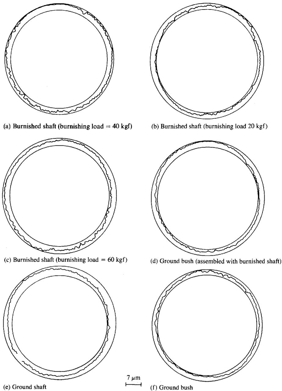
**Fig. 5** Typical roundness profiles of bushes and shafts used for load testing
