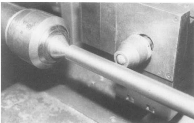
Fig. 3 Set-up showing the burnishing tool and the workpiece
