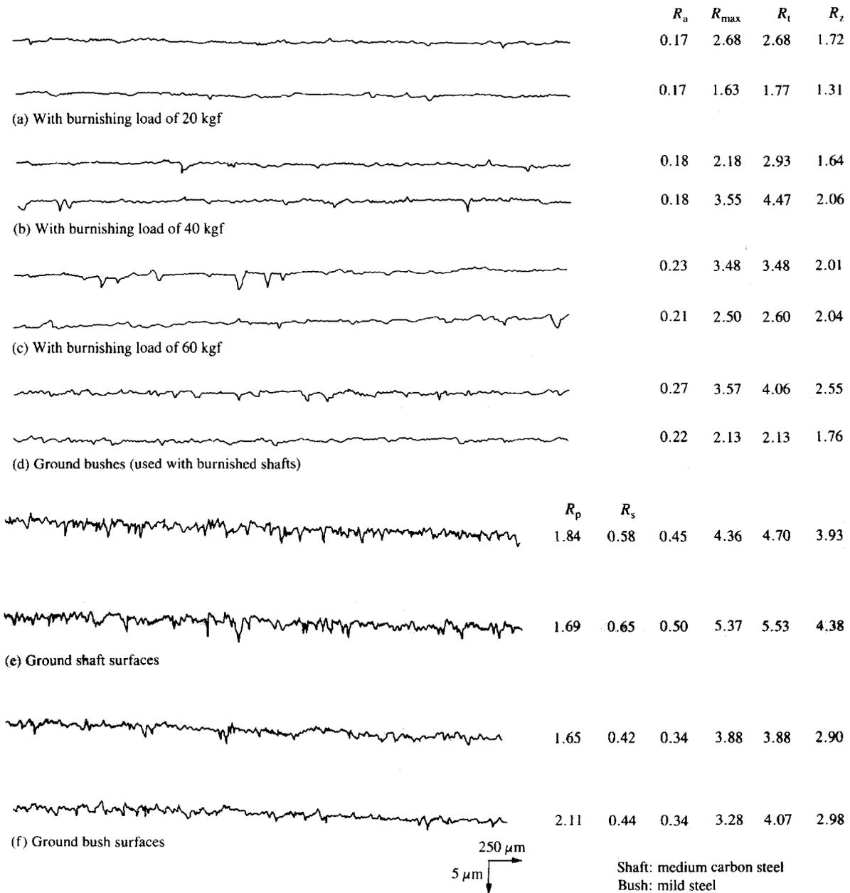
Fig. 2 Typical surface profiles of components used for load testing
