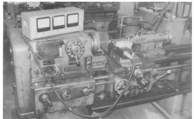
Fig. 4 Set-up showing lathe with dynamometer used for burnishing the shafts
