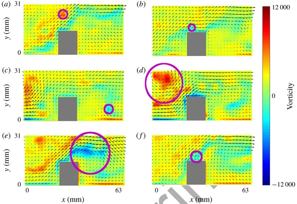
FIGURE 8. (Colour online) (a–f) Instantaneous velocity vector fields during thermoacoustic instability ( $\phi = 0.63$ ) overlaid on the field of vorticity. We can observe the emergence of a large vortex upstream of the bluff body larger than the vortices observed during the periodic epochs of intermittency. These images correspond to the same conditions as figure 7.
