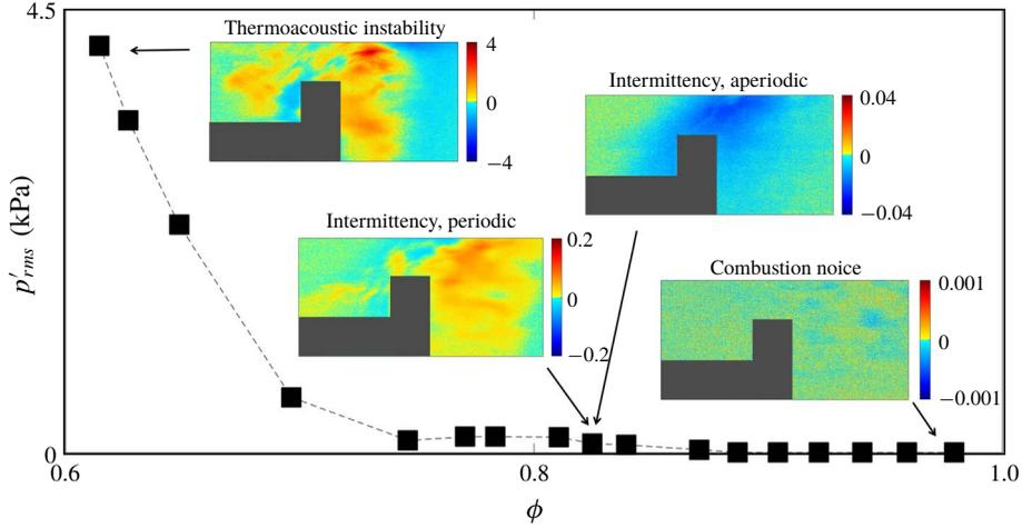
FIGURE 13. (Colour online) The variation in the  $p'_{rms}$  with respect to the equivalence ratio. The insets are instantaneous fields of local acoustic power production for the corresponding equivalence ratio. This figure shows the emergence of the self-organized coherent regions in the field of acoustic power on varying  $\phi$ . We observe the increase in size and strength of  $p'\dot{Q}'$  with a decrease in  $\phi$ .
