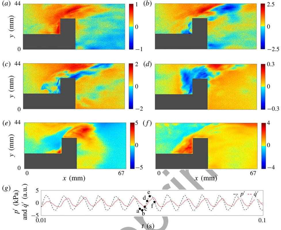
FIGURE 7. (Colour online) (a–f) Instantaneous fields of local acoustic power production  $p'Q'(x, y, t)$  at different instants of time ( $t$ ) during the occurrence of thermoacoustic instability for one periodic cycle. (g) Simultaneous  $p'(t)$  and  $q'(t)$  (obtained from PMT). Here, we observe that the fields of  $p'Q'(x, y, t)$  comprise of regions of coherent dynamics.
