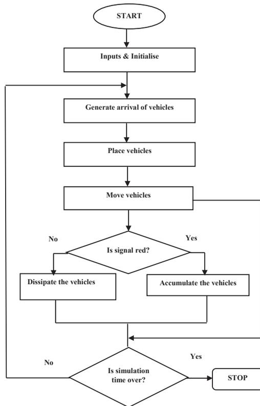
Fig. 1 Overview of the Simulation Framework
