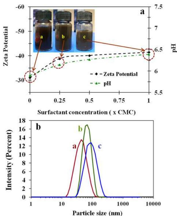
FIG. 2. (a) Zeta potential and pH variation with surfactant concentration for CuO based nanofluids. The fluids represented in the inset are: a-CuO nanofluid, b-CuO and 0.25 CMC SDS, c-CuO and 1.0 CMC SDS. (b) Particle size analysis intensity versus particle size curve for the above three fluids.
