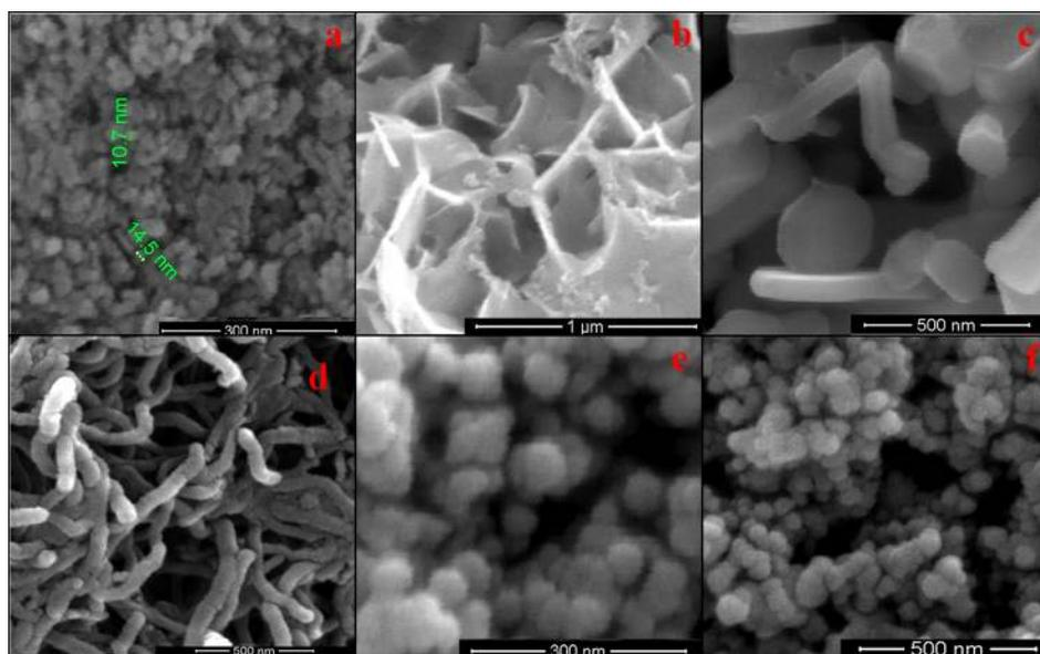
FIG. 1. (a) HRSEM image of  $\text{Al}_2\text{O}_3$  with a spherical morphology of  $\sim 13$  nm, (b)  $\text{Bi}_2\text{O}_3$  nanoparticles showing the flake morphology with a flake width of  $\sim 20$  nm, (c) ZnO nanostructures with a hexagonal rod structure with an average dimension of  $\sim 80$  nm, (d) HRSEM characterization of MWCNTs, (e) HRSEM characterization of  $\text{SiO}_2$ , and (f) HRSEM characterization of CuO (30 nm) nanoparticles.
