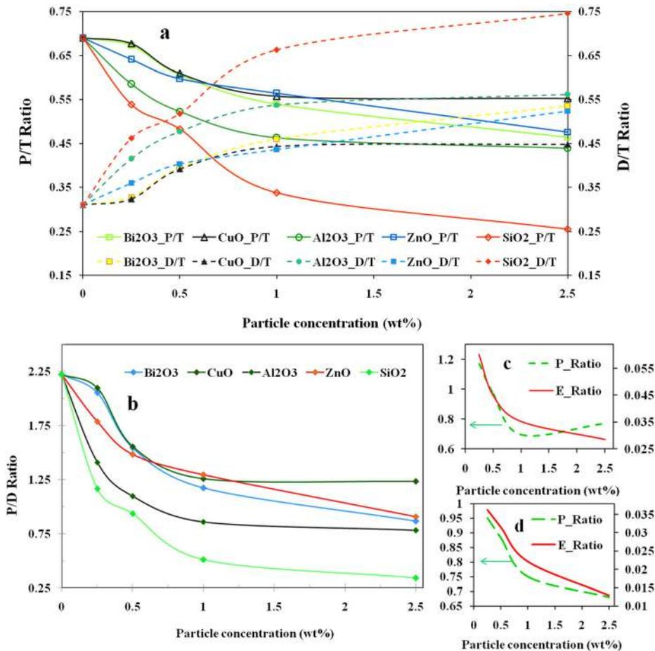
FIG. 5. (a) Variation of polar and dispersive components of surface tension to total surface tension of various nanofluids at different particle concentrations. (b) Variation of polar to dispersive components of surface tension at different particle concentrations for different nanofluids. (c) and (d) Electrical conductivity ratio (E\_Ratio) and polar component ratio (P\_Ratio) of nanofluids to that of water for CuO and Al<sub>2</sub>O<sub>3</sub> nanoparticles based nanofluids, respectively.
