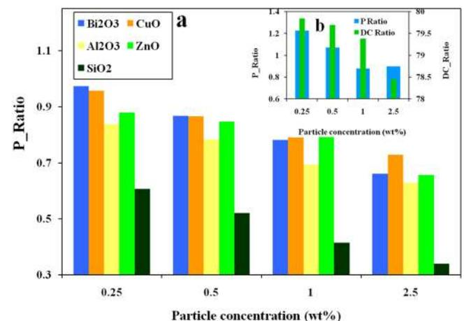
FIG. 6. (a) Variation of the ratio of the polar component of different nano-fluids to the polar component of water (P\_Ratio) with particle concentration and (b) variation of the P\_Ratio and the ratio of dielectric constant of nano-fluids to that of water (DC\_Ratio) with particle concentration.
