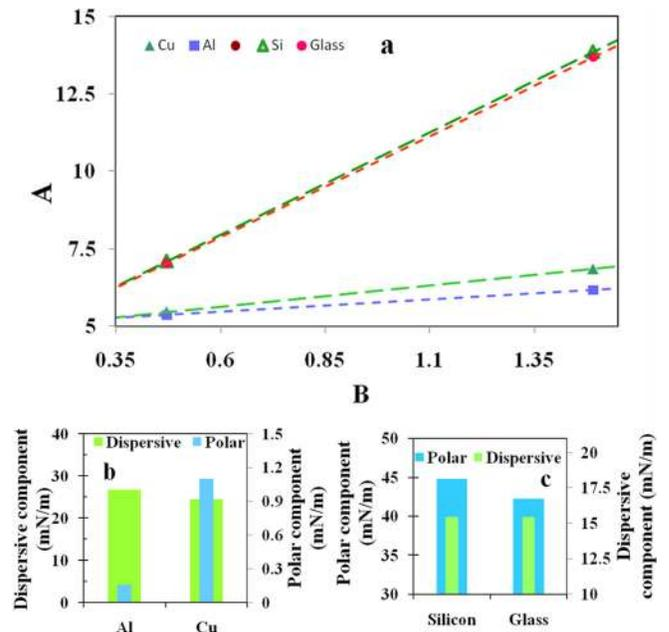
FIG. 3. (a) Linear fit for extracting polar and dispersive components; (b) polar and dispersive components for aluminium and copper substrates (c) and for silicon and glass.
