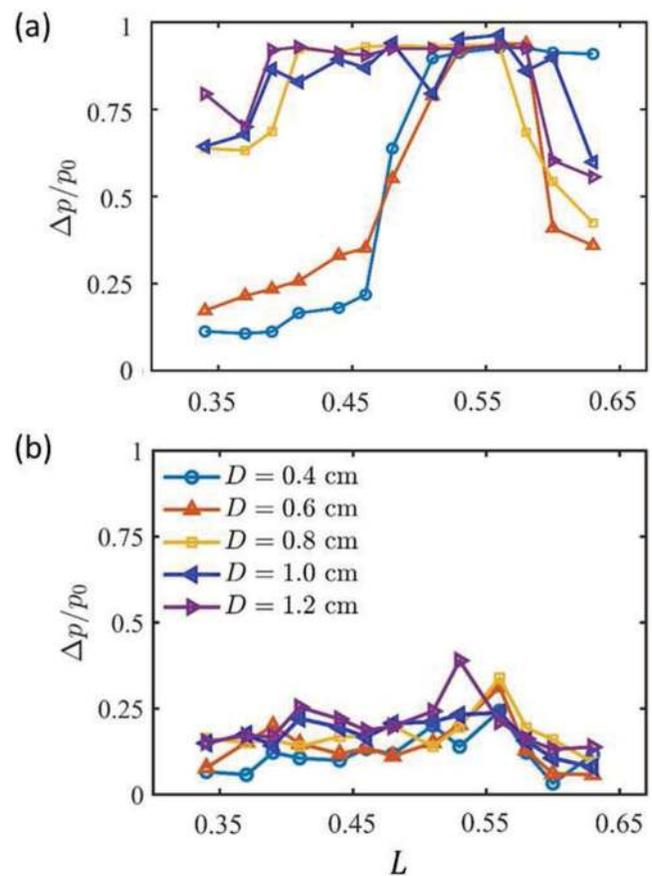
**FIG. 3.** The variation of relative suppression in the amplitude of acoustic pressure oscillations ( $\Delta p/p_0$ ) in oscillator A is plotted with respect to the length of the connecting tube ( $L$ ), for various values of diameter ( $D$ ). The amplitude of uncoupled oscillations,  $p_0$ , is 40 Pa in (a) and 120 Pa in (b). A similar trend can be observed in the case of oscillator B.
