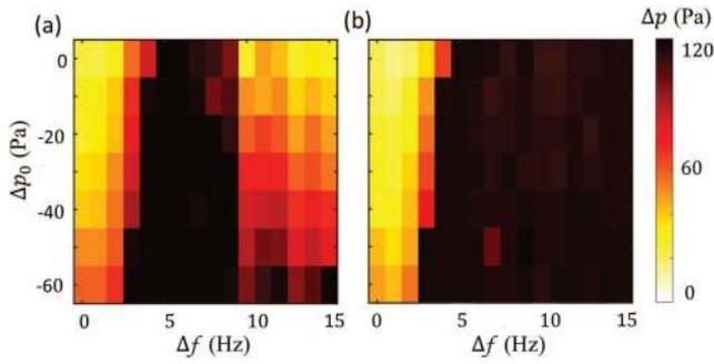
**FIG. 6.** Two-parameter bifurcation plots showing the effect of variation in amplitude mismatch,  $\Delta p_0$  and frequency detuning,  $\Delta f$  between the Rijke tube oscillators (a) A and (b) B on their oscillation quenching behavior ( $\Delta p$ ). The values of  $L$  and  $D$  are fixed at 0.48 and 1.0 cm, respectively.
