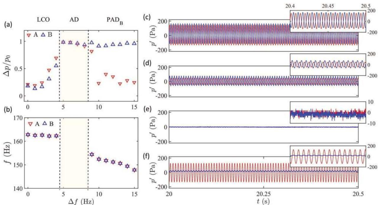
**FIG. 4.** Variation of (a) relative suppression in the response amplitudes and (b) dominant frequencies of oscillators A and B after coupling for different values of frequency detuning,  $\Delta f$ , when  $L = 0.48$ ,  $D = 1.0$  cm, and  $p_0 = 120$  Pa. The time series corresponding to various states of coupled dynamics observed for frequency detuning of (c) 0 Hz—no suppression, (d) 4.0 Hz—significant suppression, (e) 7.0 Hz—amplitude death, and (f) 15.0 Hz—partial amplitude death.
