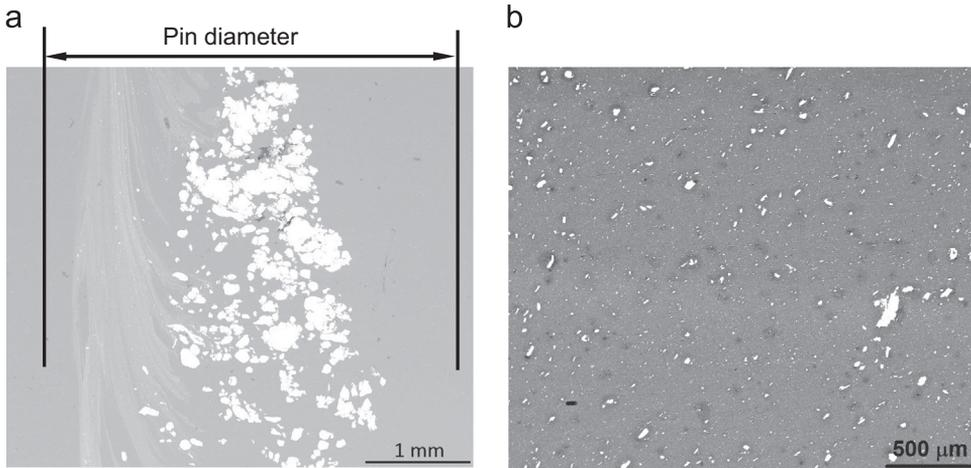
**Fig. 2.** SEM micrographs showing particle distribution of (a) coarse (70  $\mu\text{m}$ ) and (b) ball milled finer (10  $\mu\text{m}$ ) particles. Rotation speed 1200 rpm and traverse speed 24 mm/min.
