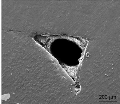
Fig. 1. SEM micrograph showing tunnel defect.
