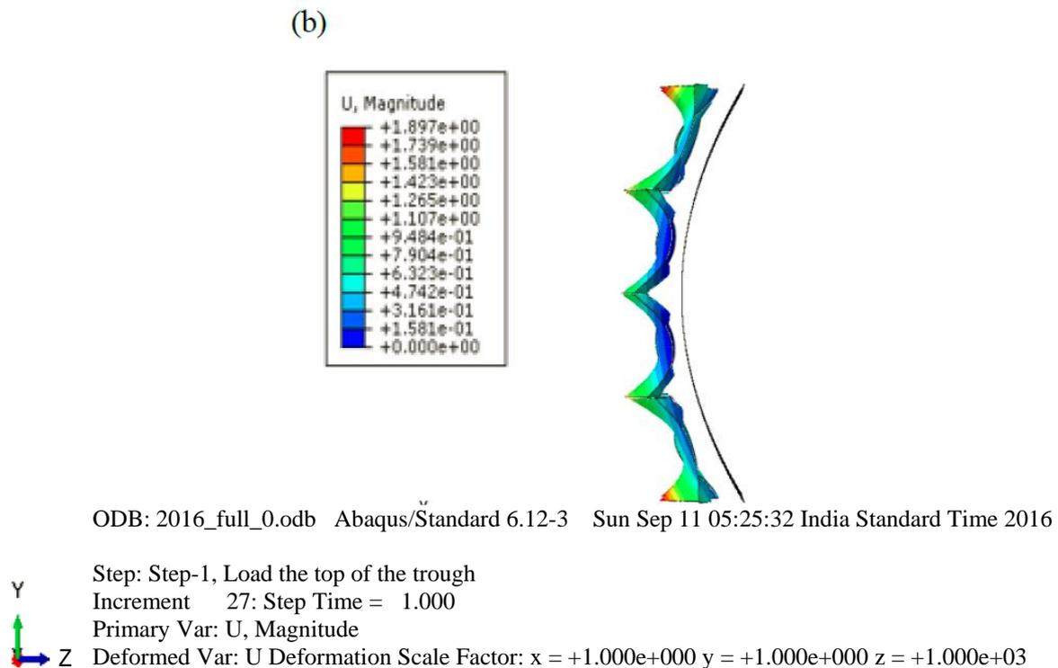
**Figure 5.** Deformation of WFRPH composite trough collector in  $0^\circ$  collector angle. (a) from its undeformed shape (superimposed) as shown in black in XZ plane (b) Trough deformation from its undeformed shape (superimposed) as shown in black in YZ plane. Color scale of deformation surface in mm, deformation scaling factor: 1000.
