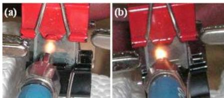
FIG. 1. (Color online) Photograph of a solid state optical switching device ( $10 \times 10 \text{ mm}^2$ ) in a (a) transparent hydrided state and (b) reflective dehydrided state.
