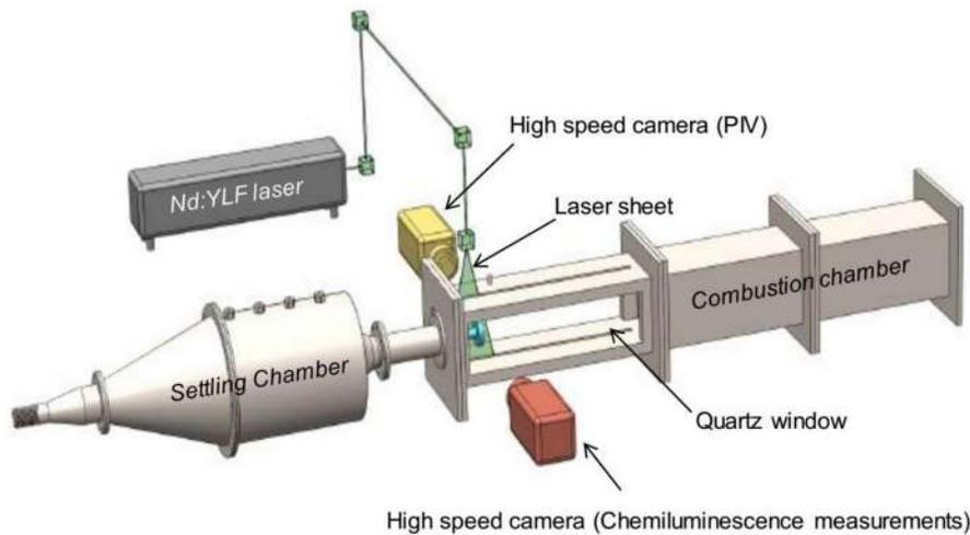
FIG. 1. The schematic of the backward facing step combustor used for the present study. A quartz window is used to facilitate high speed flame imaging and PIV. The design of the combustor was adapted from Ref. 53.
