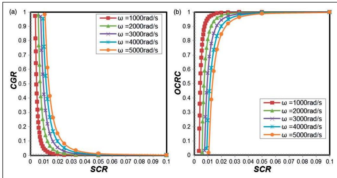
**Figure 10.** Non-dimensional (a) centrifugal growth and (b) operating clearance as a function of seal inner radius for an initial clearance of 2.5 mm at different angular speeds.
