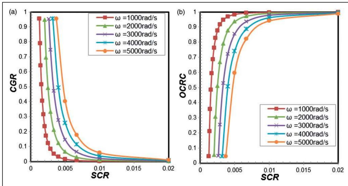
**Figure 8.** Non-dimensional (a) centrifugal growth and (b) operating clearance as a function of seal inner radius for an initial clearance of 0.5 mm at different angular speeds.
