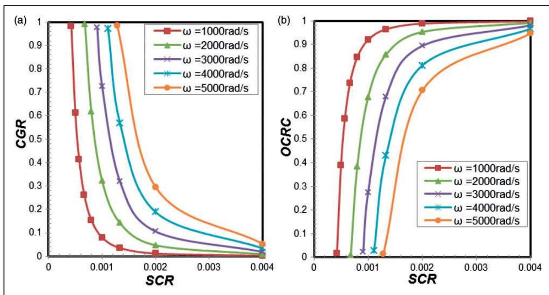
**Figure 7.** Non-dimensional (a) centrifugal growth and (b) operating clearance as a function of seal inner radius for an initial clearance of 0.1 mm at different angular speeds.
