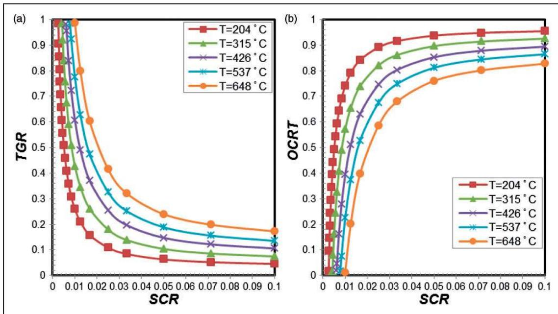
**Figure 14.** Non-dimensional (a) thermal growth and (b) operating clearance as a function of seal inner radius for an initial clearance of 2.5 mm at different temperature conditions.
