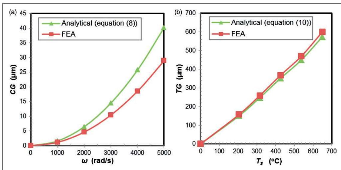
**Figure 4.** FEA versus analytical-based radial growth prediction for  $R = 50$  mm (fix-free edge conditions) as a function of (a) speed (b) temperature.
