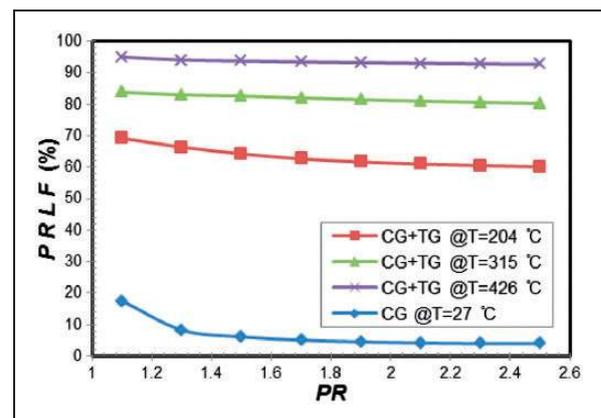
**Figure 17.** Effect of radial growth on leakage at  $\omega = 3000\text{ rad/s}$ , as function of temperature and  $PR$ .
