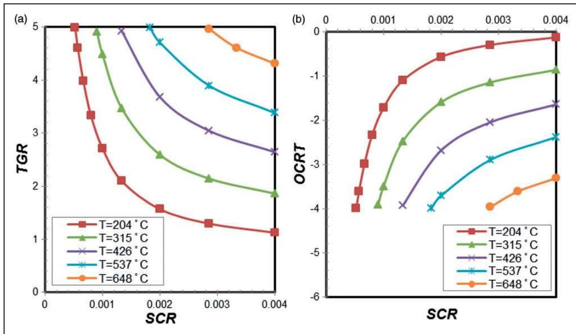
**Figure 11.** Non-dimensional (a) thermal growth and (b) operating clearance as a function of seal inner radius for an initial clearance of 0.1 mm at different temperature conditions.
