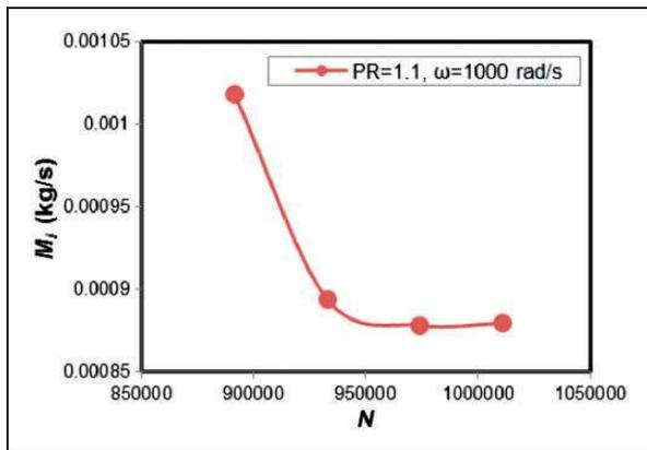
**Figure 6.** CFD grid independence study for  $R = 50$  mm and  $C = 0.1$  mm.
