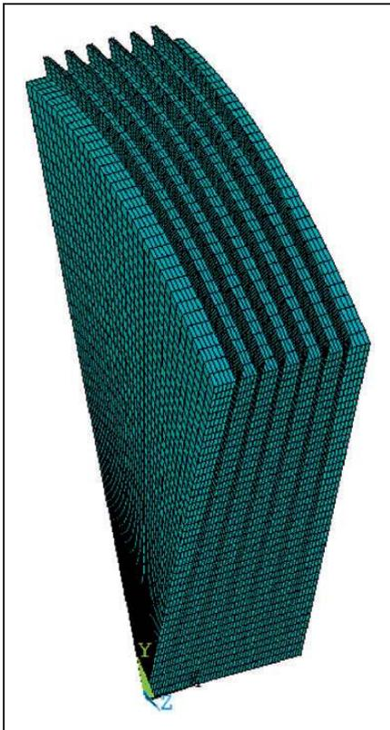
Figure 2. Three-dimensional FE mesh for rotor:  $R = 350$  mm.
