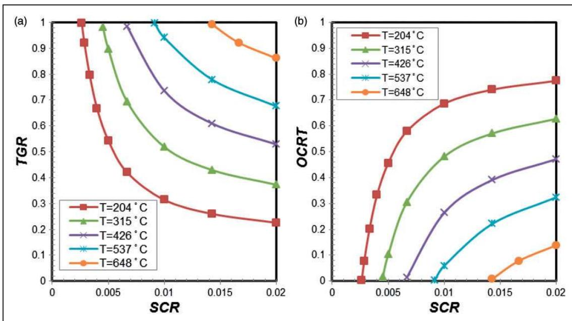
**Figure 12.** Non-dimensional (a) thermal growth and (b) operating clearance as a function of seal inner radius for an initial clearance of 0.5 mm at different temperature conditions.
