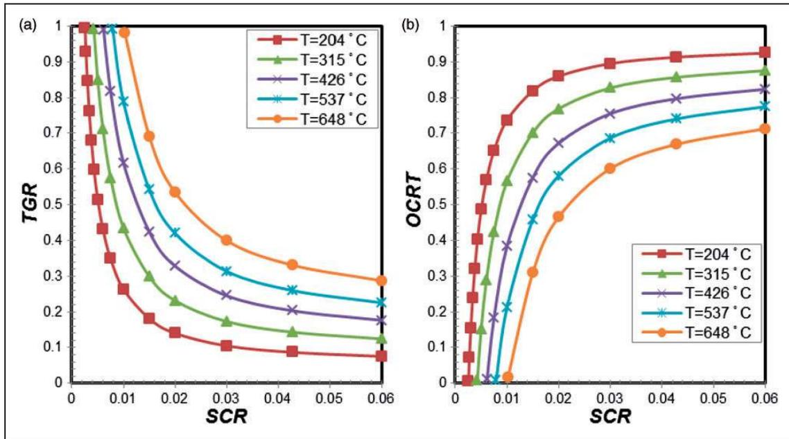
**Figure 13.** Non-dimensional (a) thermal growth and (b) operating clearance as a function of seal inner radius for an initial clearance of 1.5 mm at different temperature conditions.
