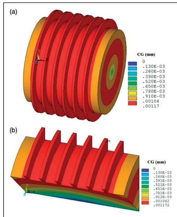
Figure 3. CG at  $\omega = 1000$  rad/s for rotor  $R = 50$  mm: (a) full 3D model (b)  $45^\circ$  sector model.
