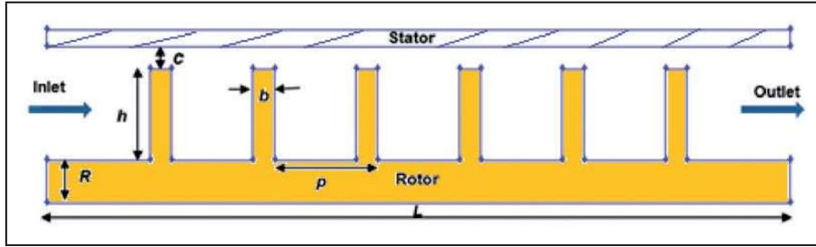
Figure 1. Schematic of GT seal (not to scale).
