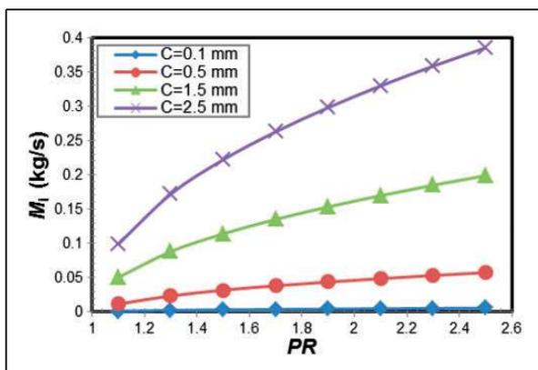
**Figure 15.** Leakage flow rate as a function of  $PR$  and initial clearance for static condition.
