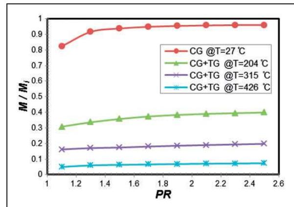
**Figure 16.** Leakage flow rate for different temperature conditions at  $\omega = 3000\text{ rad/s}$ , incorporating radial growth for seal with  $R = 50\text{ mm}$  and  $C = 0.5\text{ mm}$ .
