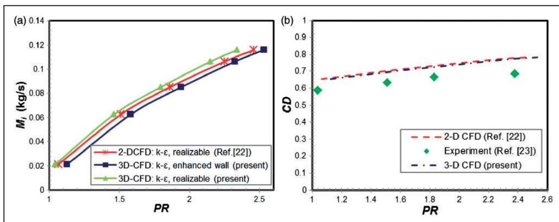
Figure 5. CFD model validation: (a) with other numerical models, (b) with experiment.
