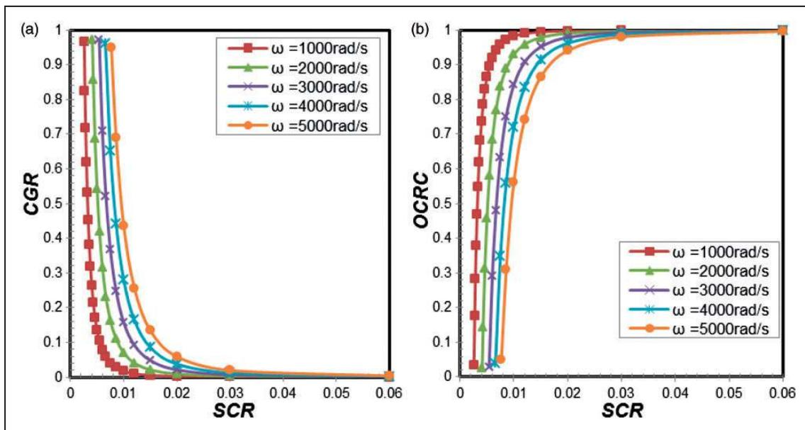
**Figure 9.** Non-dimensional (a) centrifugal growth and (b) operating clearance as a function of seal inner radius for an initial clearance of 1.5 mm at different angular speeds.
