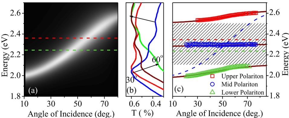
FIG. 3. (a) Mapped dispersion of the bare ASP mode. (b) Transmission spectra of the ASP-exciton hybrid system for the angle of incidence from  $30^\circ$  to  $60^\circ$ . (c) Mapped peak position showing the dispersion of the ASP-exciton hybrid modes. Dashed lines show the uncoupled mode dispersion. The brown curve shows the fit using the coupled mode model.
