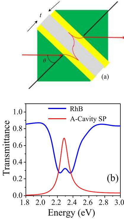
FIG. 2. (a) Schematic of the photon tunneling based configuration. (b) Transmittance of Rhodamine B (blue curve) and the ASP mode. The latter is measured using the tunnel configuration.
