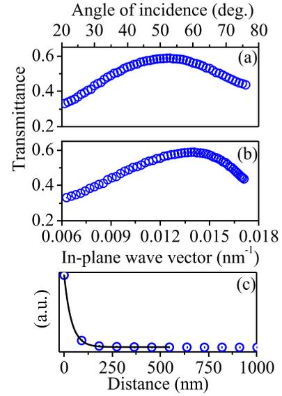
FIG. 4. (a) and (b) The measured transmittance of the middle mode (transmittance at 2.29 eV) as a function of the angle of incidence and in-plane wave vector, respectively. (c) Inverse Fourier transform of (b), showing the spatial profile of the middle mode.
