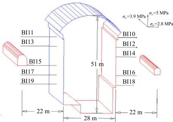
Fig. 7. Outline of the cavern and locations of multi-point borehole extensometer for the cavern of Shiobara hydropower station.
