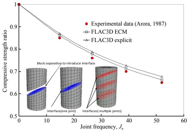
Fig. 6. Variation of compressive strength ratio ( $\sigma_{cr}$ ) with joint frequency ( $J_n$ ) for Jamrani sandstone having  $90^\circ$  joint inclination.
