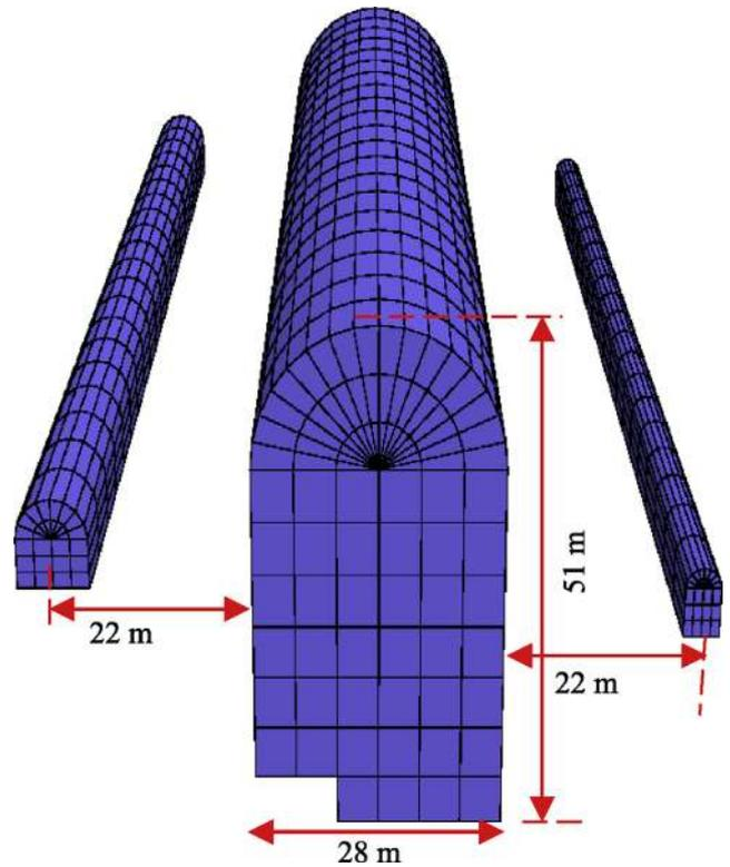
Fig. 8. FLAC3D model of Shiobara powerhouse cavern: underground openings.
