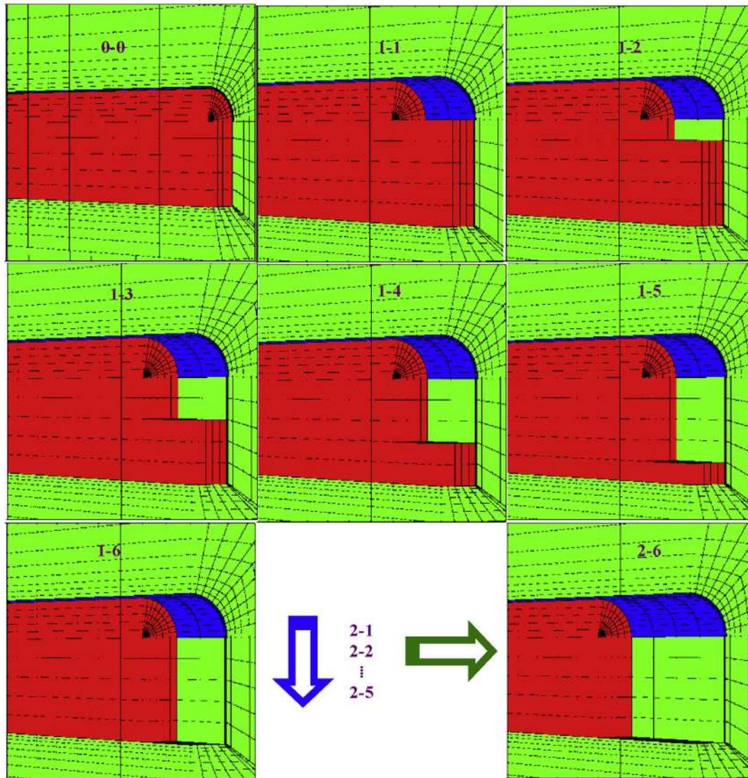
Fig. 10. Complete excavation scheme using null model available in FLAC3D.
