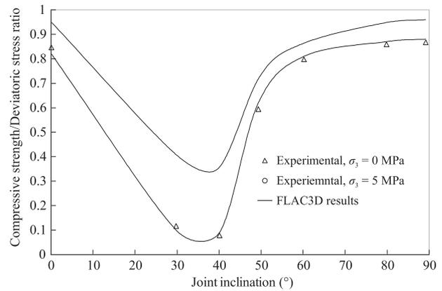
Fig. 5. Variation of deviatoric stress ratio with joint inclination for Jamrani sandstone with a single joint.
