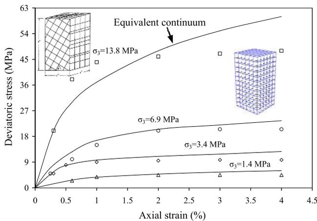
Fig. 4. Comparison of equivalent continuum modelling results with those from experiments (Brown and Trollope, 1970) for 60°/30° block jointed specimens at four different confining pressures (Sitharam et al., 2007).
