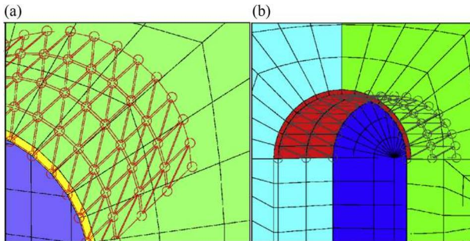
Fig. 12. Close-up view of the cavern face with supports of (a) concrete liner, and (b) shotcrete (after first stage of excavation).
