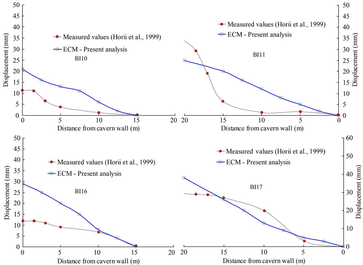
Fig. 11. Comparison of relative displacements along the measurement lines.
