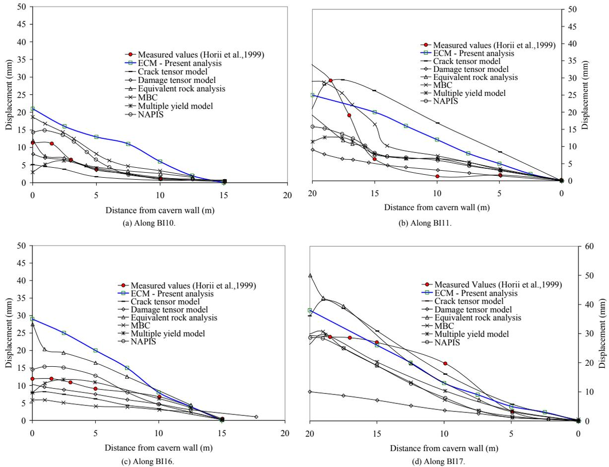
**Fig. 13.** Comparisons of relative displacements along different measurement lines.
