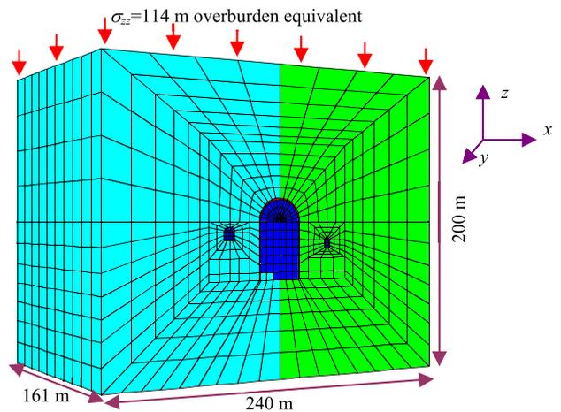
Fig. 9. FLAC3D mesh of Shiobara hydropower cavern with complete boundaries.
