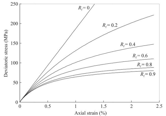
Fig. 1. Dependency of nonlinearity in the stress–strain behaviour on the failure ratio ( $R_f$ ).
