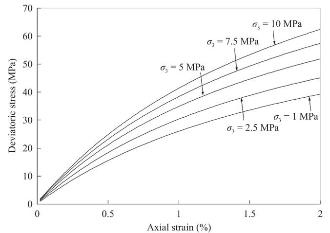
Fig. 2. Influence of confining stress on the stress–strain behaviour.
