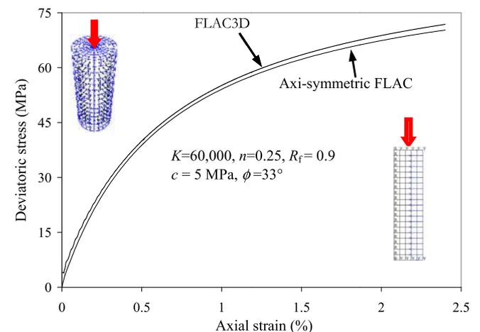
Fig. 3. Stress–strain curves obtained from numerical tests with those from FLAC3D and axi-symmetric FLAC.
