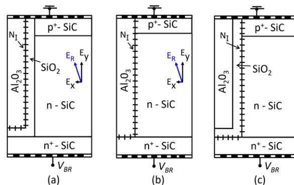
Fig.1. (a) Cross-section of the unit cell of the proposed Charge-Sheet Super Junction [1]. Diagram not to scale; the actual SiO<sub>2</sub> liner is much thinner than shown. (b) A variation of (a) with SiO<sub>2</sub> liner removed. (c) A variation of (a) with the negative interface charge  $N_I$  moved to the SiO<sub>2</sub>/SiC interface.
