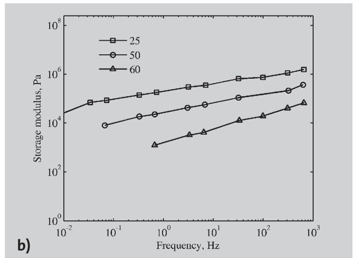
**Figure 6:** Comparison of the frequency dependence of the moduli at different temperatures (parameters as given in Table 1, Asphalt 1): (a) Model results, (b) Experimental data trends.
