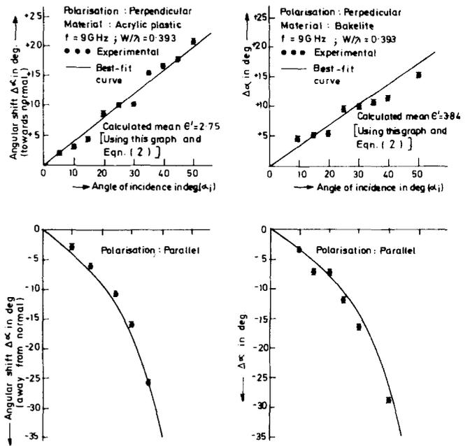
FIG. 3. Angular beam-shift versus angle of incidence.
