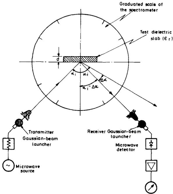
FIG. 2. Angular beam-shift measurement.
