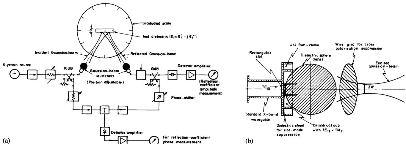
FIG. 1. X-band beam-wave spectrometer and the Gaussian-beam launcher.
