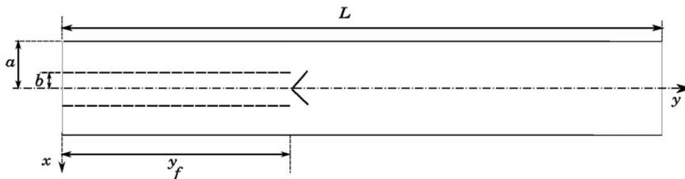
**Figure 22.** Geometry of coupled system with an axisymmetric wedge flame stabilized on a wire. Here,  $L$  is the length of the duct,  $(b/a)$  is the ratio of burner to duct radius and  $\tilde{y}_f$  is the flame location along the length of the duct. Figure reproduced with permission from Subramanian and Sujith.<sup>39</sup>
