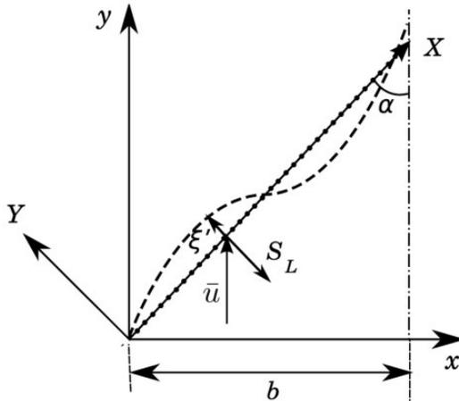
**Figure 21.** Geometry of an axisymmetric wedge flame stabilized on a wire. Here  $\xi'$  is the displacement of instantaneous flame shape from the unperturbed flame shape along  $X$ ,  $\alpha$  is the flame angle,  $S_L$  is the laminar flame speed,  $b$  is the radius of the burner, and  $\bar{u}$  is the mean flow. Figure reproduced with permission from Subramanian and Sujith.<sup>39</sup>
