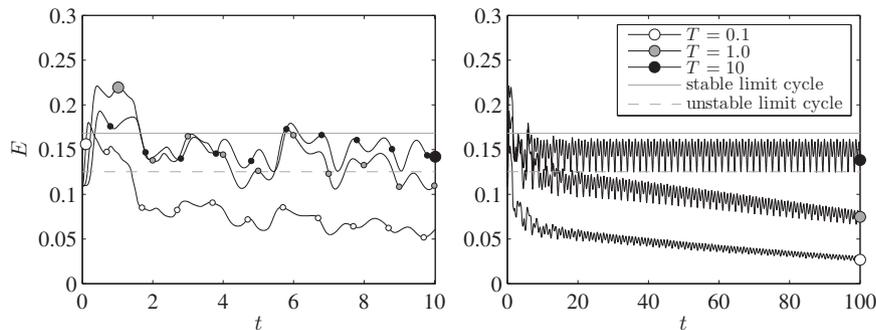
**Figure 20.** Energy,  $E$ , as a function of time,  $t$ , for the three initial states in Figure 19. The optimal initial state with  $T = 10$  has smaller transient growth at short times but then grows to the stable limit cycle (not shown).
