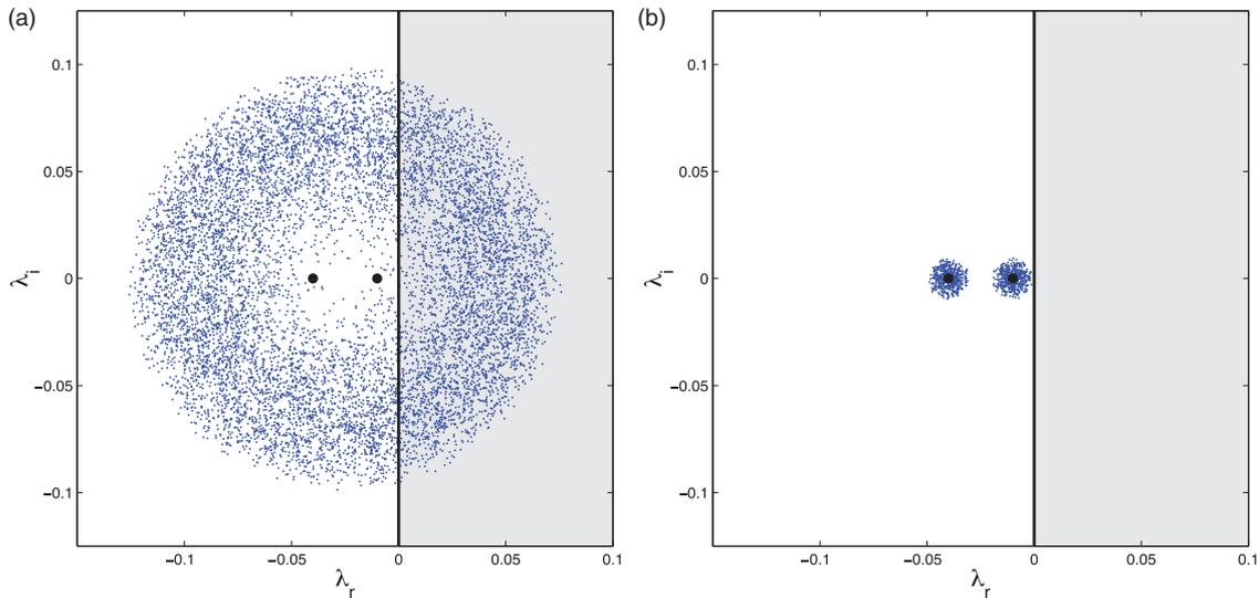
**Figure 6.** Sensitivity of eigenvalues for (a) the non-normal system at  $Re = 50$ , and (b) the normal system (with zero off-diagonal term) at the same Reynolds number. In both cases, the matrix  $A$  has been perturbed by random matrices of norm  $10^{-2}$ .
