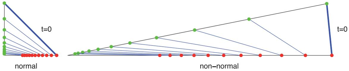
**Figure 3.** Geometric sketch of energy growth/decay in a two-dimensional orthogonal (left) and nonorthogonal (right) system. In either case, the two vector components contract, ultimately yielding a solution vector of zero length. In the normal case, monotonic decay toward a zero-length solution is observed; in the non-normal case, transient growth prevails before the asymptotic limit of a zero-length vector is reached.
