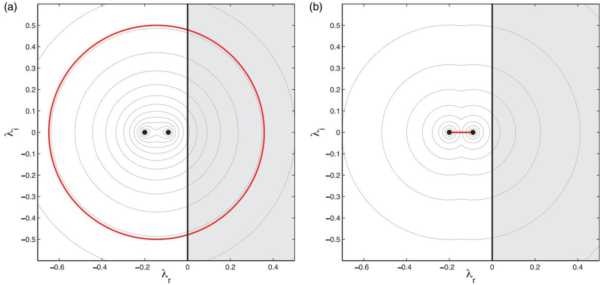
**Figure 4.** (a) Boundary of the numerical range (in red) and spectrum (in black symbols) of the non-normal matrix  $A$  for  $Re = 10$ . (b) Boundary of the numerical range (in red) and spectrum (in black symbols) of  $A$  when the off-diagonal term is set to zero, thus rendering  $A$  a normal matrix.
