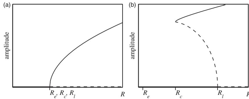
**Figure 1.** The steady state oscillation amplitude,  $a_{SS}$ , as a function of a control parameter,  $R$ , for (a) a supercritical bifurcation and (b) a subcritical bifurcation.  $R_l$  is the point at which the fixed point (i.e., the zero amplitude solution) becomes unstable.  $R_c$  is the point below which no oscillations can be sustained and  $R_e$  is the point below which all perturbations decrease monotonically to zero.
