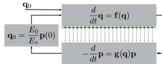
**Figure 8.** Sketch of iterative optimization scheme based on the nonlinear, direct and variable-coefficient, adjoint governing equations, derived from a variational framework. The checkpoints at which the direct solutions are stored are indicated by green symbols.
