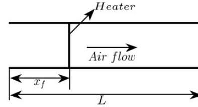
Figure 9. Diagram of a horizontal Rijke tube.
