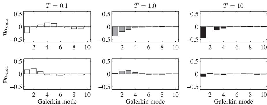
**Figure 19.** Initial states that give maximum transient growth at  $E_0 = 0.1099$  for  $T = 0.1$ ,  $T = 1.0$ , and  $T = 10$ . The optimal initial state with  $T = 10$  has most energy in the first mode and appreciable energy in the third and fourth modes.
