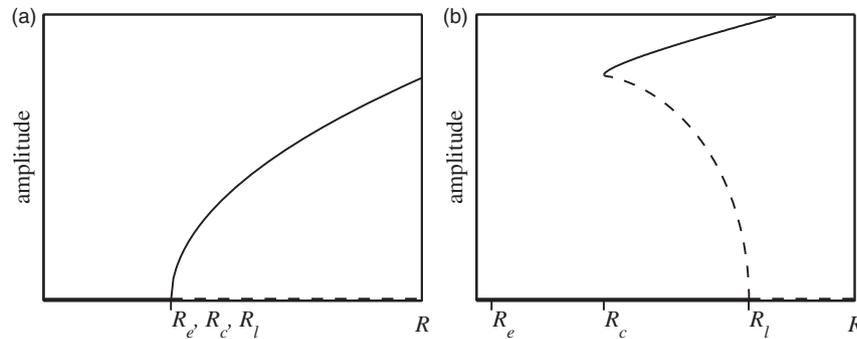
**Figure 1.** The steady state oscillation amplitude,  $a_{SS}$ , as a function of a control parameter,  $R$ , for (a) a supercritical bifurcation and (b) a subcritical bifurcation.  $R_l$  is the point at which the fixed point (i.e., the zero amplitude solution) becomes unstable.  $R_c$  is the point below which no oscillations can be sustained and  $R_e$  is the point below which all perturbations decrease monotonically to zero.
