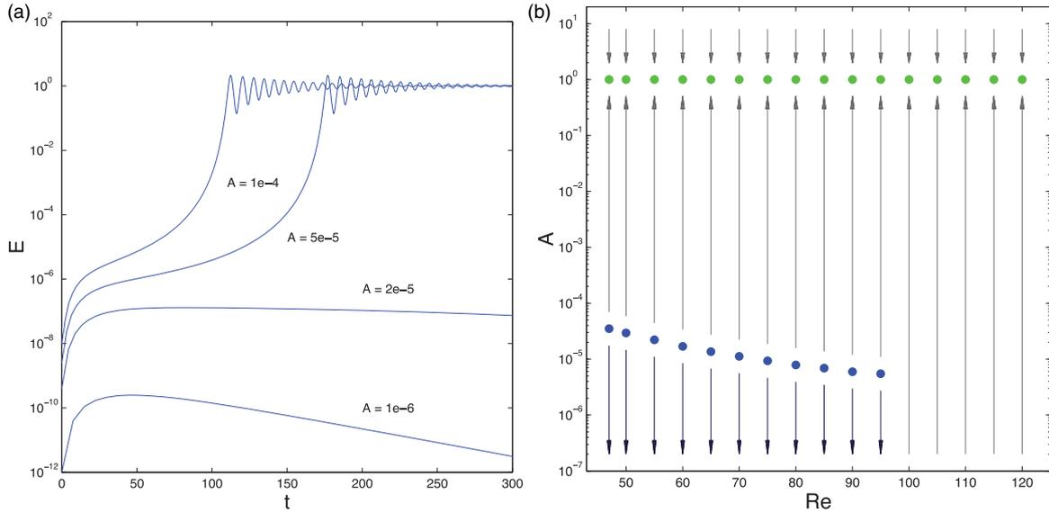
**Figure 5.** (a) Perturbation energy versus time for the nonlinear system (equation (9)) starting with  $\mathbf{q}_0 = A(0, 1)^T$  and four different amplitudes  $A$ . (b) Bifurcation diagram for the nonlinear system (equation (9)), indicating the triggering amplitudes (blue symbols) and the nonlinear steady state (green symbols). The critical Reynolds number is  $Re_{crit} = 100$ .
