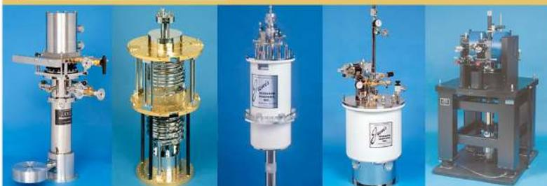
10 mK to 800 K      LHe/LN<sub>2</sub> Cryostats
