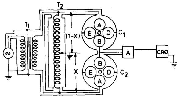
FIG. 2. Circuit arrangement;  $T_1$ —isolating transformer,  $T_2$ —8-decade inductive voltage divider, A—amplifier, CRO—oscilloscope detector,  $C_{12}$ ,  $C_2$ —right hand and left hand cross capacitors.
