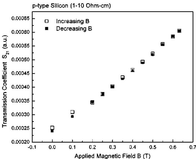
FIG. 3. Variation of the transmission coefficient with respect to the applied magnetic field for a *p*-type silicon semiconductor sample.
