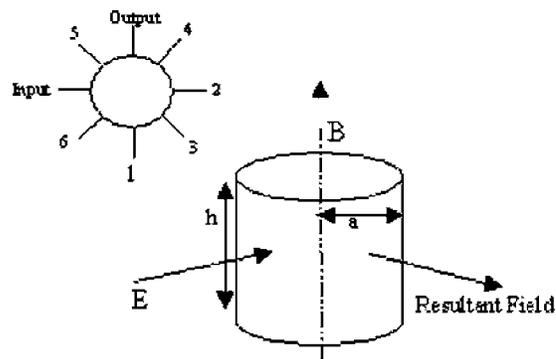
FIG. 1. Schematic diagram of the TE<sub>112</sub> cylindrical bimodal cavity.
