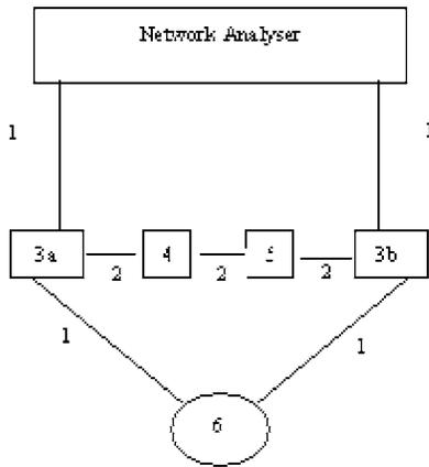
FIG. 2. Experimental arrangement of the microwave Hall effect technique.
