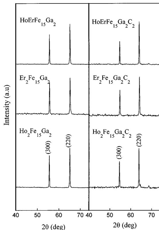
FIG. 3. X-ray diffractograms of magnetically aligned  $(\text{Ho}_{1-x}\text{Er}_x)_2\text{Fe}_{15}\text{Ga}_2\text{C}_y$  ( $x=0, 0.5, 1$ , and  $y=0, 2$ ) at room temperature.
