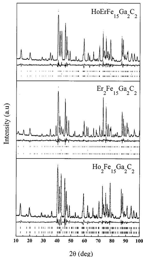
FIG. 2. Neutron diffraction patterns of  $(\text{Ho}_{1-x}\text{Er}_x)_2\text{Fe}_{15}\text{Ga}_2\text{C}_2$  ( $x=0, 0.5,$  and  $1$ ) at room temperature. The points and the curve refer to the recorded pattern and the calculated fit, respectively. A difference pattern is plotted in the lower part of the figure. The first and third sets of bars refer to the nuclear and magnetic diffraction peaks. The second set refer to  $\alpha$ -Fe as impurity.
