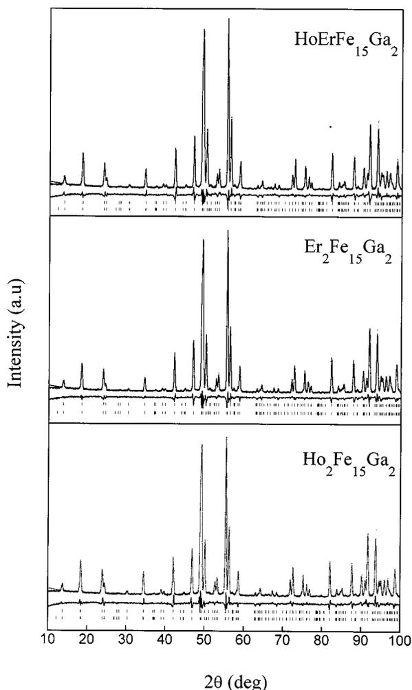
FIG. 1. Neutron diffraction patterns of  $(\text{Ho}_{1-x}\text{Er}_x)_2\text{Fe}_{15}\text{Ga}_2$  ( $x=0, 0.5,$  and  $1$ ) at room temperature. The points and the curve refer to the recorded pattern and the calculated fit, respectively. A difference pattern is plotted in the lower part of the figure. The first and second sets of bars refer to the nuclear and magnetic diffraction peaks.
