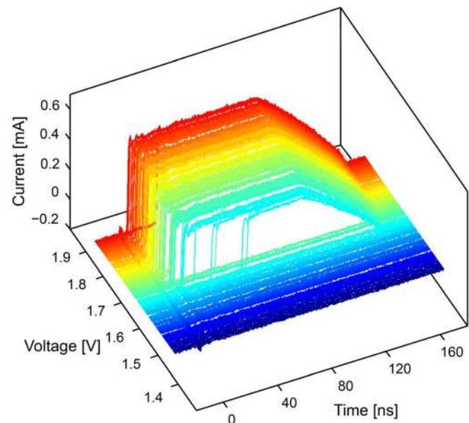
FIG. 2. Time-resolved measurement of the device current  $I_d$  for voltage pulses ranging from  $1.40$  to  $1.85\text{ V}$ . The overlay of  $I_d$  reveals the dependency of transient parameters such as delay time on the voltage pulse. The height of the applied voltage pulse is color coded. This viewgraph demonstrates the pronounced dependence of the delay time upon the height of the voltage pulse.
