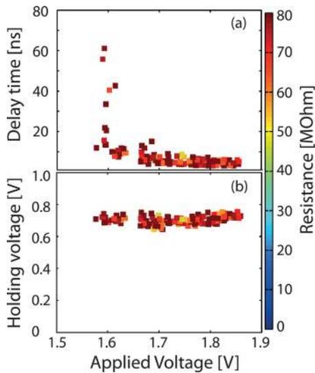
FIG. 3. Dependence of delay time  $t_d$  (a) and holding voltage  $V_h$  (b), on the applied voltage. The different colors represent the device resistance before the threshold switching event.
