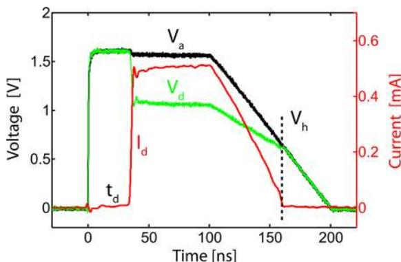
FIG. 1. Time-resolved measurement of threshold switching characteristics of  $\text{GeTe}_6$  device for the applied voltage pulse  $V_a$  of  $1.60\text{ V}$  ( $1\text{ ns}$  rise time,  $100\text{ ns}$  plateau time and trailing edge, respectively) (black color), as well as the measured device voltage  $V_d$  (green color) and the device current  $I_d$  (red color).  $V_h$  denotes the holding voltage below which the device returns to the high resistance *off* state.
