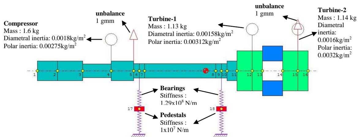
**Figure 1.** Rotor system schematic
