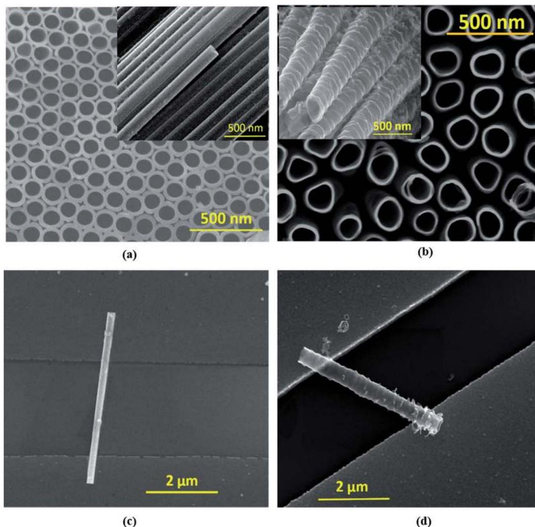
Fig. 1 FESEM image showing the top and side view (inset) of (a) EGNT and (b) DMTNT and (c) and (d) show the individual TiO<sub>2</sub> nanotube devices of EGNT and DMTNT, respectively, on Au electrodes on top of the SiO<sub>2</sub>/Si substrate.
