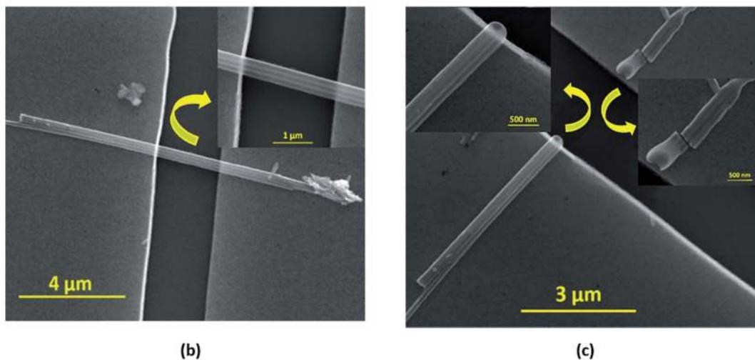
Fig. 9 (a) In the 'Model C' breakdown, the  $J$ - $V$  curve displays mixed features of nonlinearity along with sudden big steps in  $J$  before the breakdown point which may be the characteristics for breaking of the bridge between the nanotubes in the bundle. SEM images exhibit a bundle of 3 EGTNT (b) before and (c) after the breakdown; magnified SEM images are also displayed in the insets.
