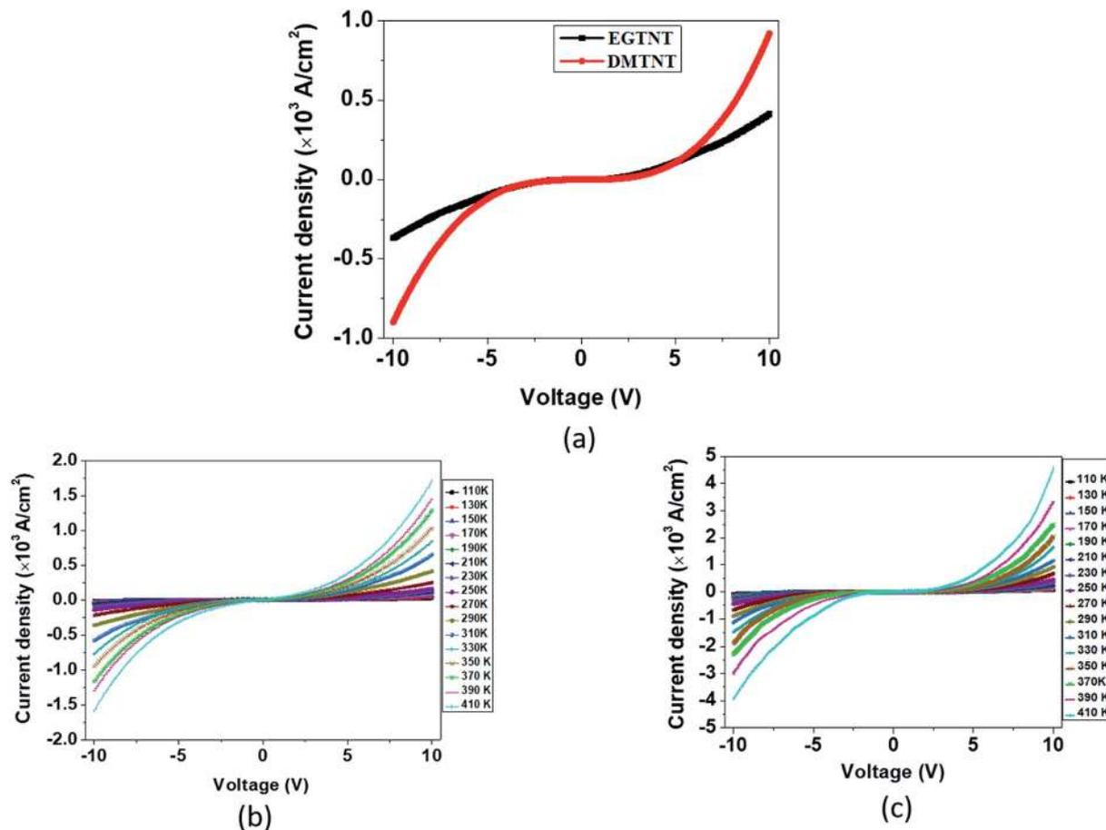
Fig. 2 Current density–voltage ( $J$ – $V$ ) plots (a) for EGTNT and DMTNT at room temperature, (b) for the individual EGTNT at different temperatures and (c) for the individual DMTNT at different temperatures.
