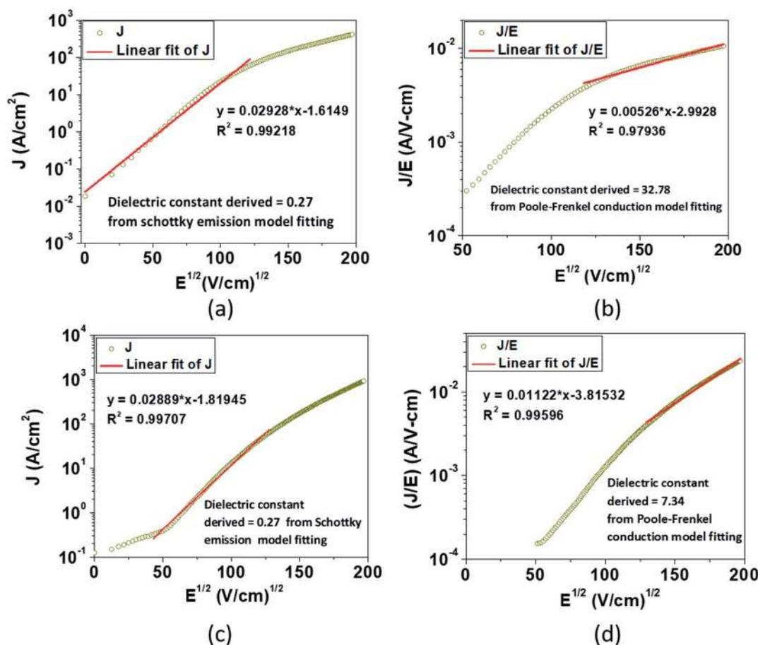
Fig. 3 The experimental semi-logarithmic plot of  $J$  vs.  $E^{1/2}$  according to eqn (1) for (a) EGTNT and (c) DMTNT at 290 K in the lower bias region; the experimental semi-logarithmic plot of  $(J/E)$  vs.  $E^{1/2}$  according to eqn (2) for (b) EGTNT and (d) DMTNT at 290 K in the higher electric field area. The red straight line denotes the fitting curve to those specified equations in a fixed range of the electric field.
