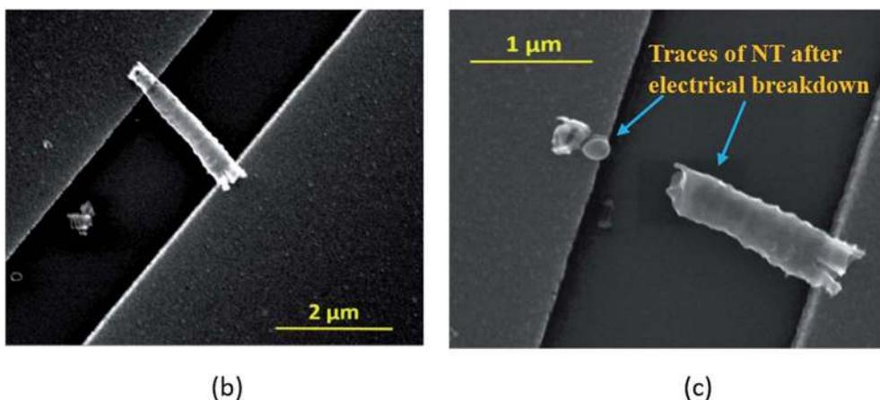
Fig. 6 (a) In the 'Model A' breakdown, the  $J$ - $V$  curve displays features of an exponential rise in  $J$  along with nonlinearity before the verge of breakdown and reveals a stepwise fall of  $J$  during the electrical breakdown. SEM images exhibit a single DMTNT (b) before and (c) after the breakdown.
