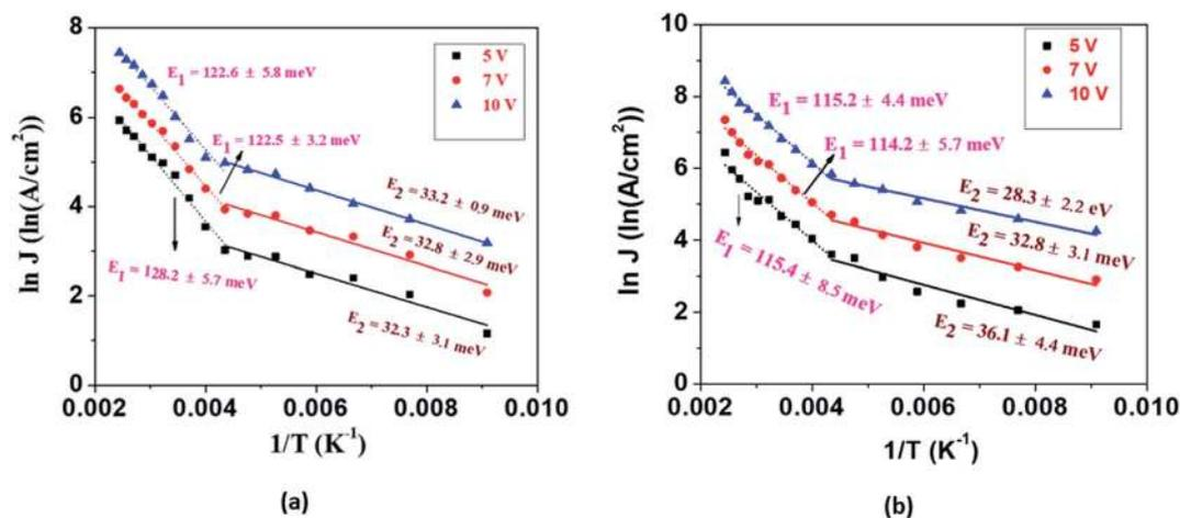
Fig. 4 Logarithm of current density ( $J$ ) as a function of the reciprocal of the temperature between 110 K and 410 K at 3 different bias voltages (a) for individual EGTNT and (b) for individual DMTNT showing intermediate deep and shallow donor levels  $E_1$  and  $E_2$ , respectively. The symbols are the experimental data and the straight lines and dotted lines are the linearly fitted curves to the data.
