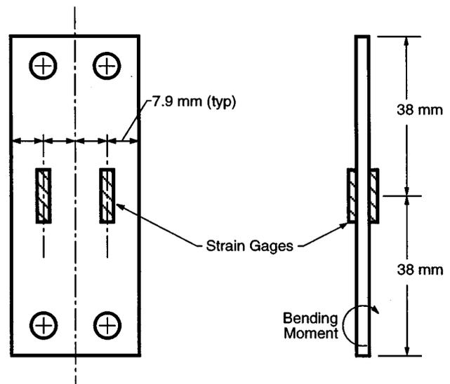
FIG. 4. Schematic of strain sensing beam.
