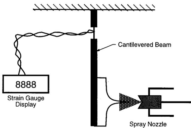
FIG. 2. Schematic of momentum rate probe.
