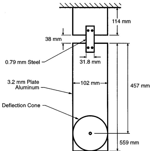
FIG. 3. Dimensions of compound cantilevered beam.
