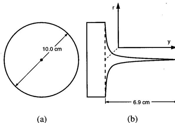
FIG. 1. Deflection cone for use with momentum rate probe: (a) front view; (b) side view.
