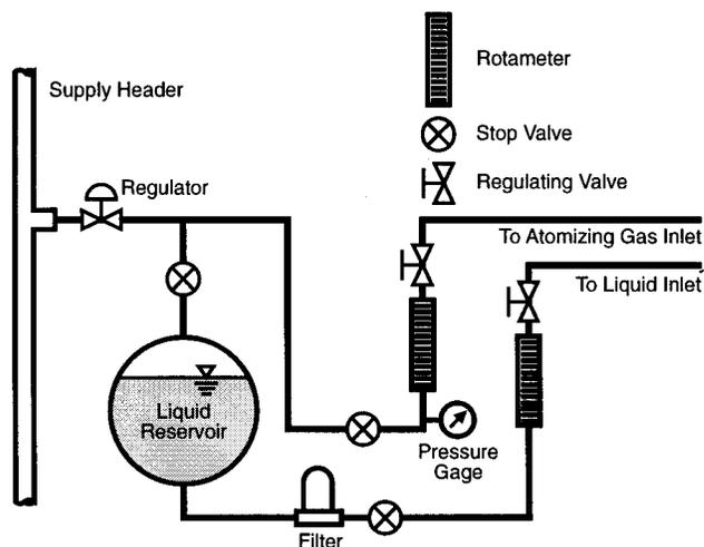
FIG. 7. Schematic of effervescent atomizer supply system.
