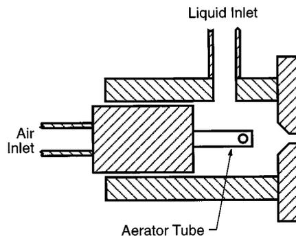
FIG. 6. Schematic of effervescent atomizer.
