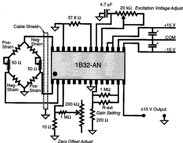
FIG. 5. Circuit diagram of strain gage bridge and signal conditioning electronics.
