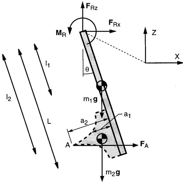
FIG. 10. Free body diagram of rigid beam and deflection cone. Note that the strain-sensing beam supplies the reaction force and moment at the top of the rigid beam.
