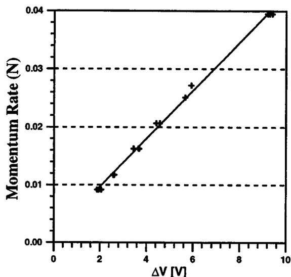
FIG. 8. Sample calibration curve for momentum rate probe.
