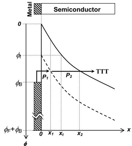
FIG. 3. Energy band diagram of a reverse biased metal semiconductor junction depicting TTT;  $\phi_t$  is the trap ionization energy,  $\phi_B$  is the barrier height, and  $\phi = \phi_F + \phi_B$  is the bottom of the conduction band in metal. Locations  $x_1$ ,  $x_2$ , and  $x_t$  are used as integration limits in TTT and DT model equations.
