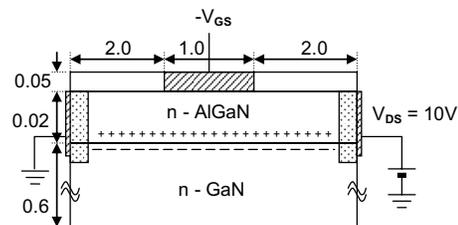
FIG. 1. AlGa<sub>x</sub>N/GaN HEMT structure with nonzero  $V_{DS}$  used in Ref. 6 for gate leakage measurements and in this work for simulation. Device dimensions are in microns. Doping in the source/drain region is assumed to be  $1 \times 10^{19}$  cm<sup>-3</sup>. Figure is not to scale.
