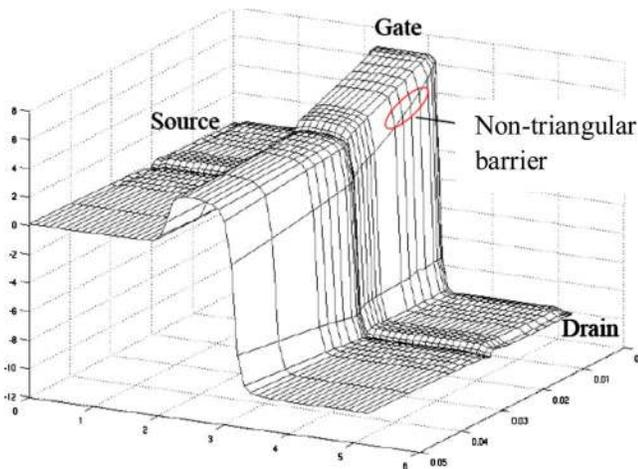
FIG. 2. (Color online) Simulated conduction band profile within the device depicting the nontriangular shape of the gate potential barrier.
