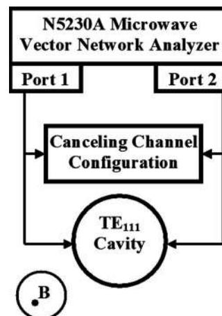
FIG. 1. Block diagram of the experimental arrangement for MFE technique.
