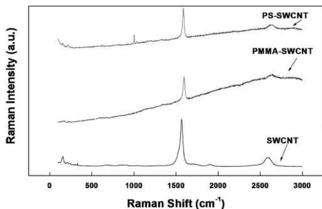
FIG. 2. Raman spectra for SWCNT, 0.5% w/w loaded SWCNT in PS and 0.5% w/w loaded SWCNT in PMMA.
