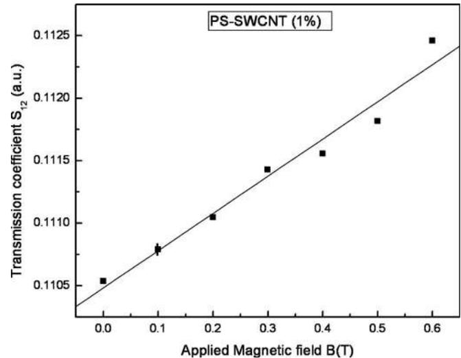
FIG. 3. Variation in transmission coefficient with respect to the applied magnetic field for the PMMA-SWCNT (1%) composites. The vertical line indicates the error in the measurement.
