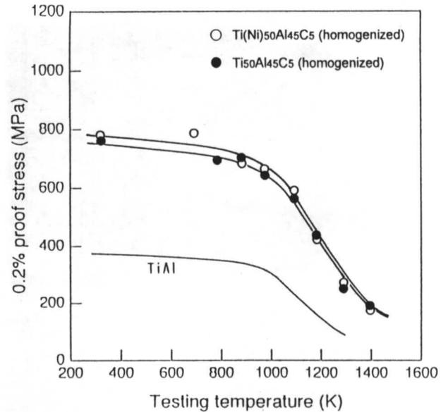
Fig.5 Compressive 0.2 % proof strength as a function of the testing temperature. Included for purpose of comparison is the proof strength of binary TiAl alloy.
