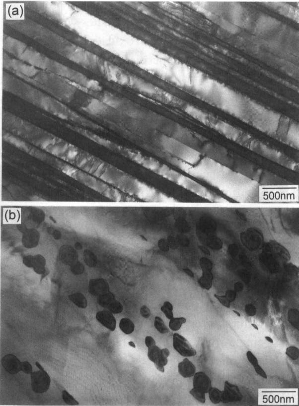
Fig.4 TEM micrographs of the composite with impurities (Ti(Ni)<sub>50</sub>Al<sub>45</sub>C<sub>5</sub>), showing smaller precipitates in place of lamellar disappeared; (a) as cast, and (b) homogenized at 1000°C.
