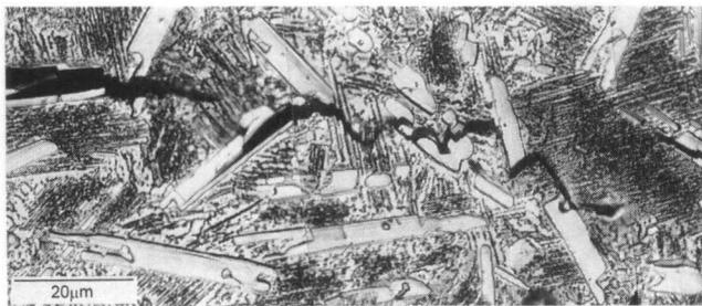
Fig.8 An optical micrograph taken at the crack tip of the composite with impurities (Ti(Ni)<sub>50</sub>Al<sub>45</sub>C<sub>5</sub>) homogenized at 1000°C.
