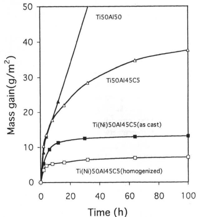
Fig.9 Mass gain curves as a function of oxidation time at 900°C in air.
