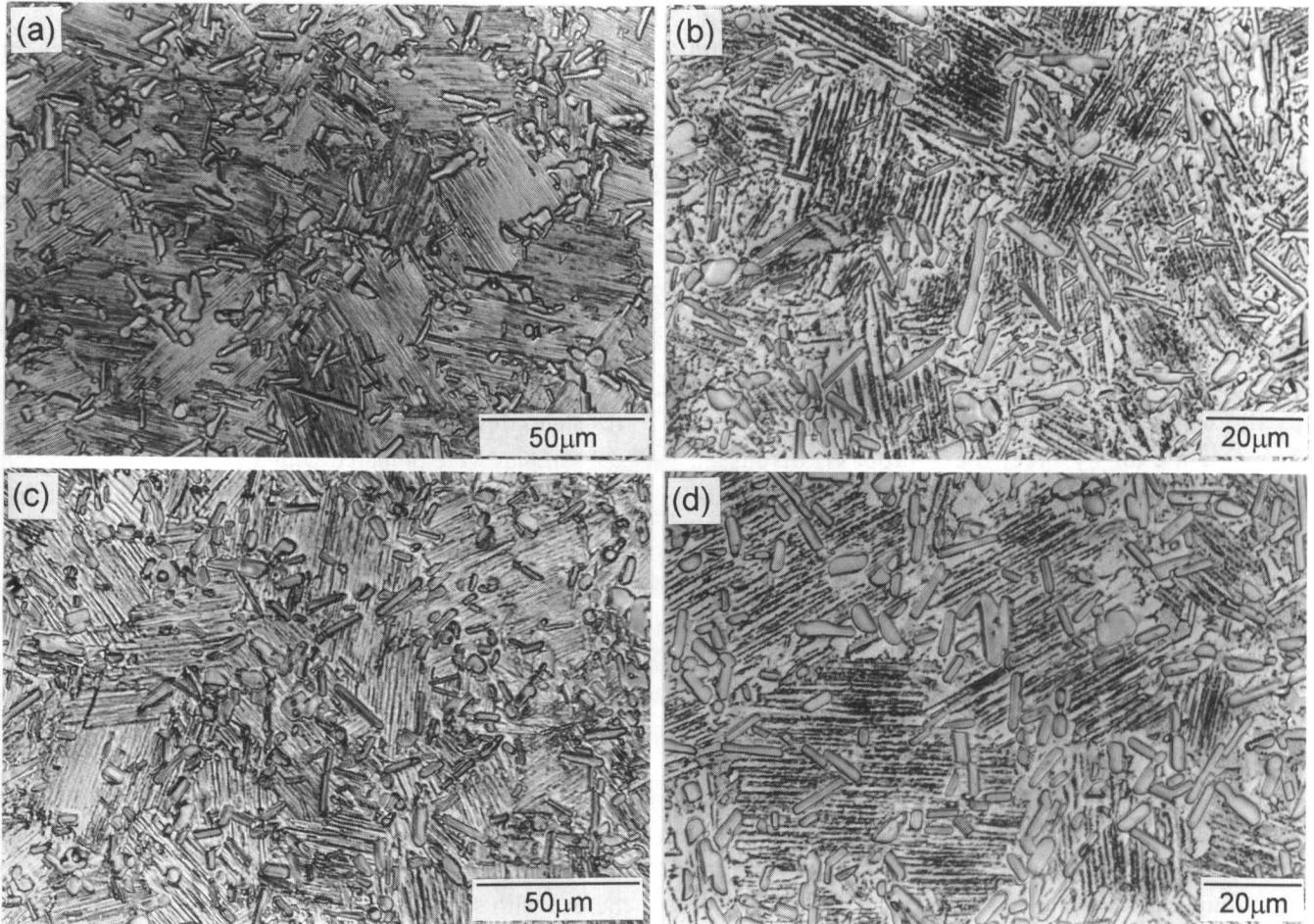
Fig.2 Optical microstructures of the arc-melted composites; (a) as cast and (b) homogenized composites without impurities ( $Ti_{50}Al_{45}C_5$ ), and (c) as cast and (d) homogenized composites with impurities ( $Ti(Ni)_{50}Al_{45}C_5$ ).
