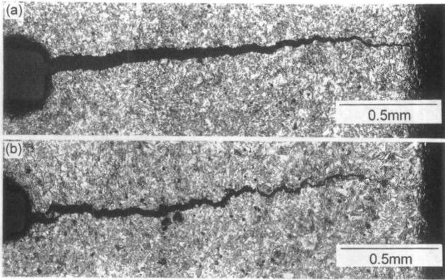
Fig.7 Optical micrographs of the fracture toughness tested composites with impurities (Ti(Ni)<sub>50</sub>Al<sub>45</sub>C<sub>5</sub>); (a) as cast, and (b) homogenized at 1000°C.
