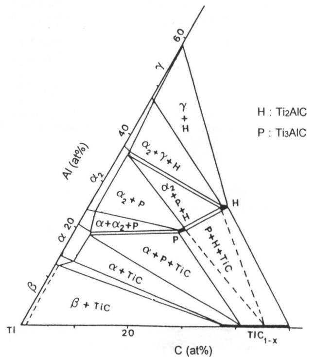
Fig.3 The phase diagram<sup>24)</sup> of Ti-Al-C ternary system at  $1050^{\circ}C$ .
