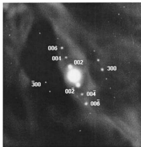
FIG. 4. Microdiffraction pattern of the agglomerated flowerlike cluster in the  $2.16 \text{ g/dm}^3$   $C_{60}$  solution microfilm.
