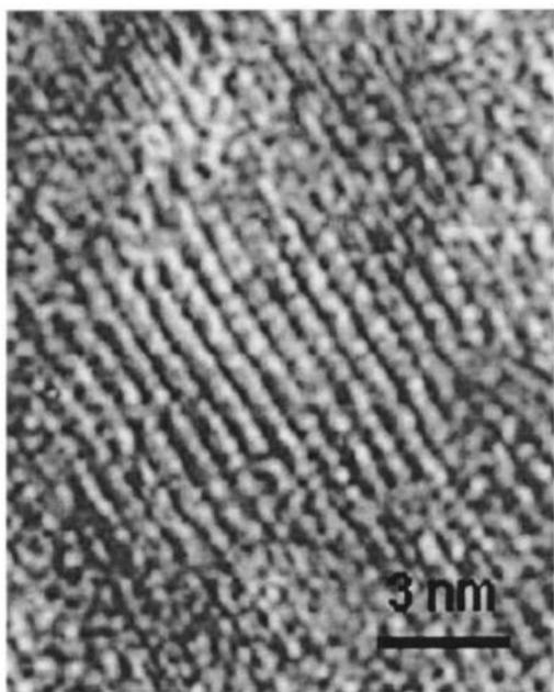
FIG. 2. HRTEM image of a fullerene monomer in the 0.02 g/dm<sup>3</sup> C<sub>60</sub> solution microfilm.
