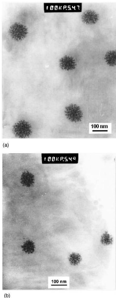
FIG. 1. (a) TEM image of the  $0.06 \text{ g/dm}^3$   $C_{60}$  solution microfilm at a higher magnification (100 K X) showing the microdomains within the spherical aggregate. (b) TEM micrograph of the  $0.36 \text{ g/dm}^3$   $C_{60}$  solution microfilm at 100 K X magnification.
