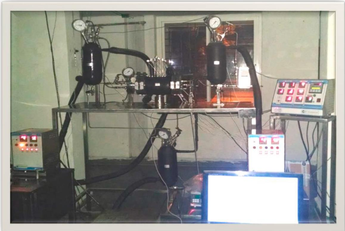
Figure A2: Bench scale high pressure continuous setup for studying methane hydrate decomposition kinetics in sub-sea environments
