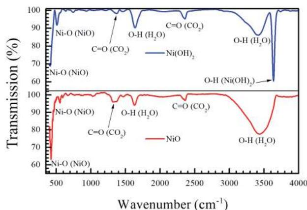
Fig. 3 Fourier-transform infrared response of the precursor  $\text{Ni}(\text{OH})_2$  and annealed NiO nanoparticles shows that the oxidation from hydroxide to oxide is complete by annealing at  $400\text{ }^\circ\text{C}$  for 2 h.
