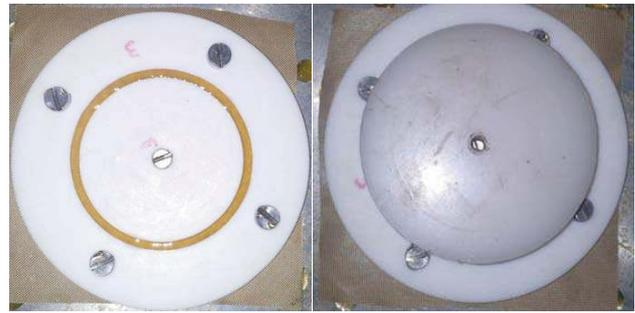
**Figure 1.** Teflon mould for a ring-shaped specimen.
