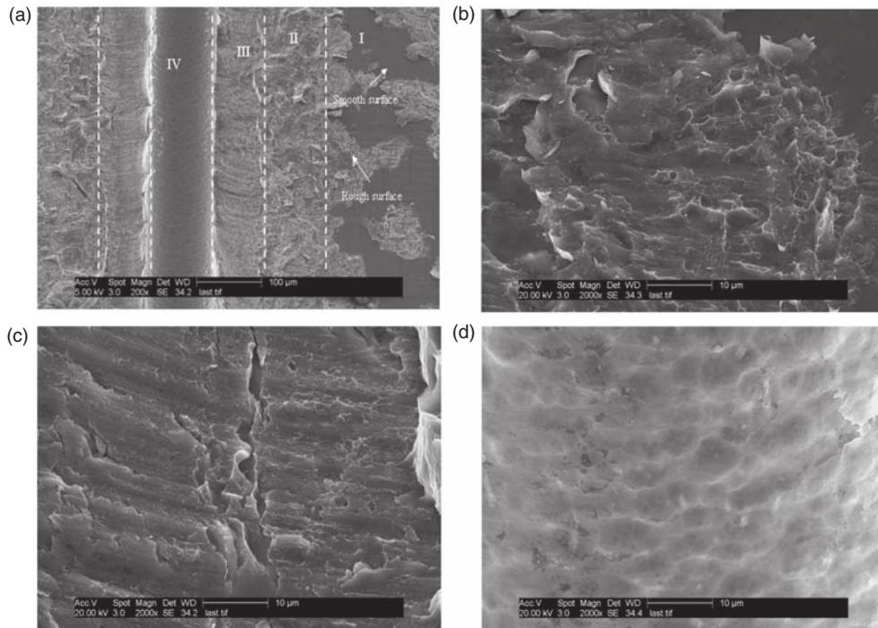
**Figure 8.** (a) Failure surface of a peel test specimen, (b) Zone I at high magnification, (c) Zone III at high magnification, and (d) Zone IV at high magnification.
