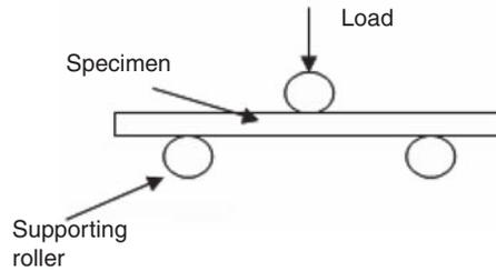
**Figure 4.** Setup for three-point bend tests.
