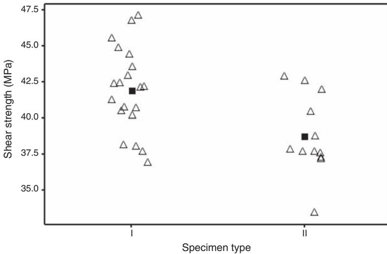
**Figure 14.** Results of three-point bend tests ( $\Delta$ : results for an individual specimen,  $\blacksquare$ : mean value for each type of specimen).
