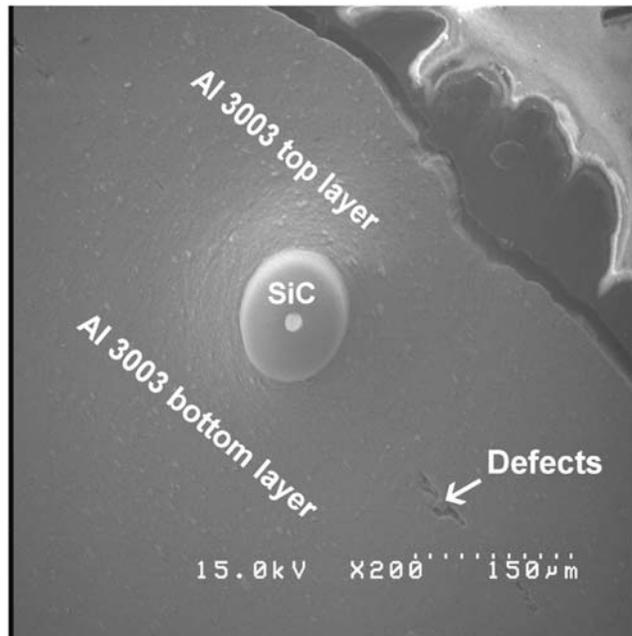
**Figure 5.** SEM picture of an embedded SiC fiber between Al 3003 foils [9].
