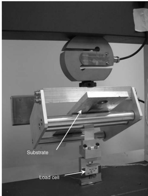
**Figure 3.** Setup for peel tests.
