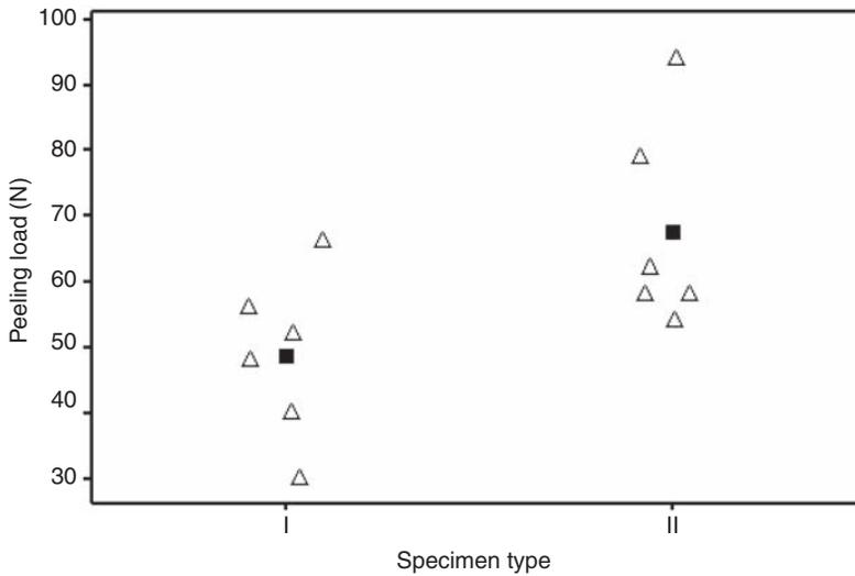
**Figure 7.** Results of peel tests ( $\Delta$ : result for an individual specimen,  $\blacksquare$ : mean value for each type of specimen).
