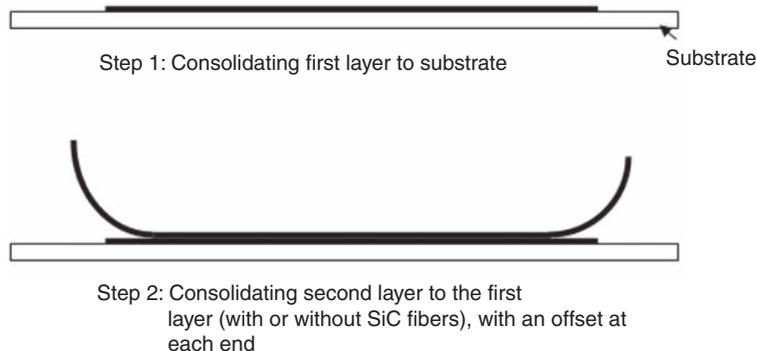
**Figure 2.** Fabrication procedure for peel test specimens.
