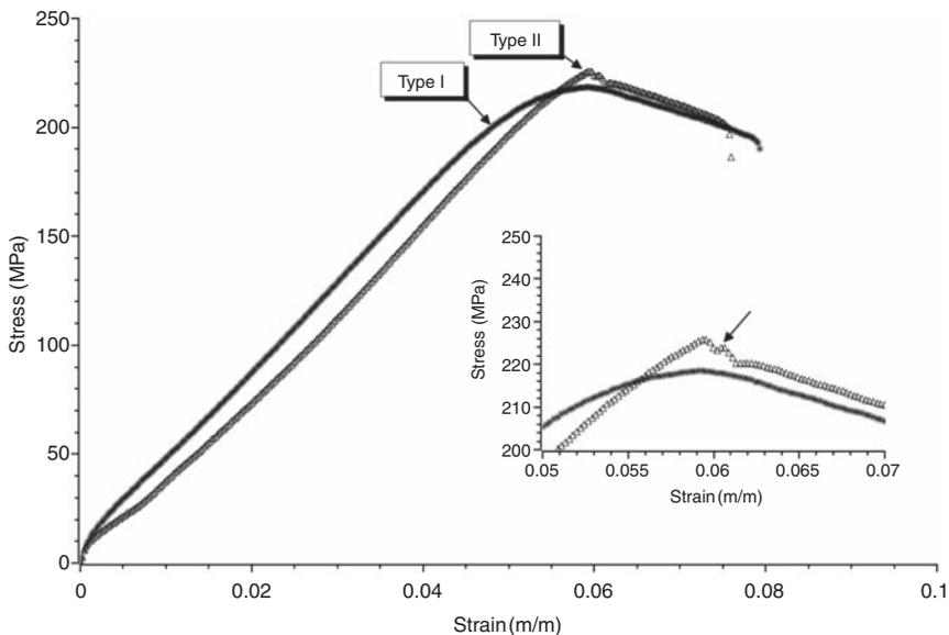
**Figure 9.** Tensile stress–strain curves of Type I and Type II specimens.
