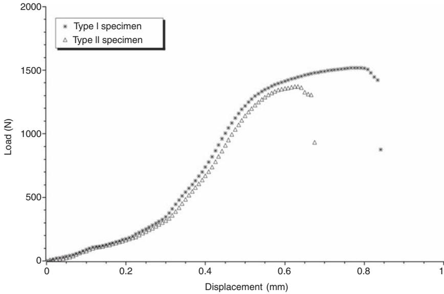
**Figure 13.** Load–displacement curves of Type I and Type II specimens obtained in three-point bend tests.
