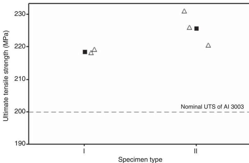
**Figure 10.** Results of tensile tests ( $\Delta$ : result for an individual specimen,  $\blacksquare$ : mean value for each type of specimen).
