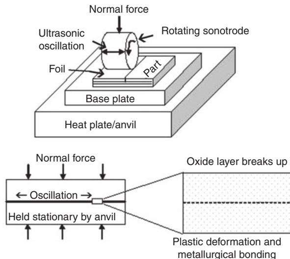
**Figure 1.** Schematic of the UC process.
