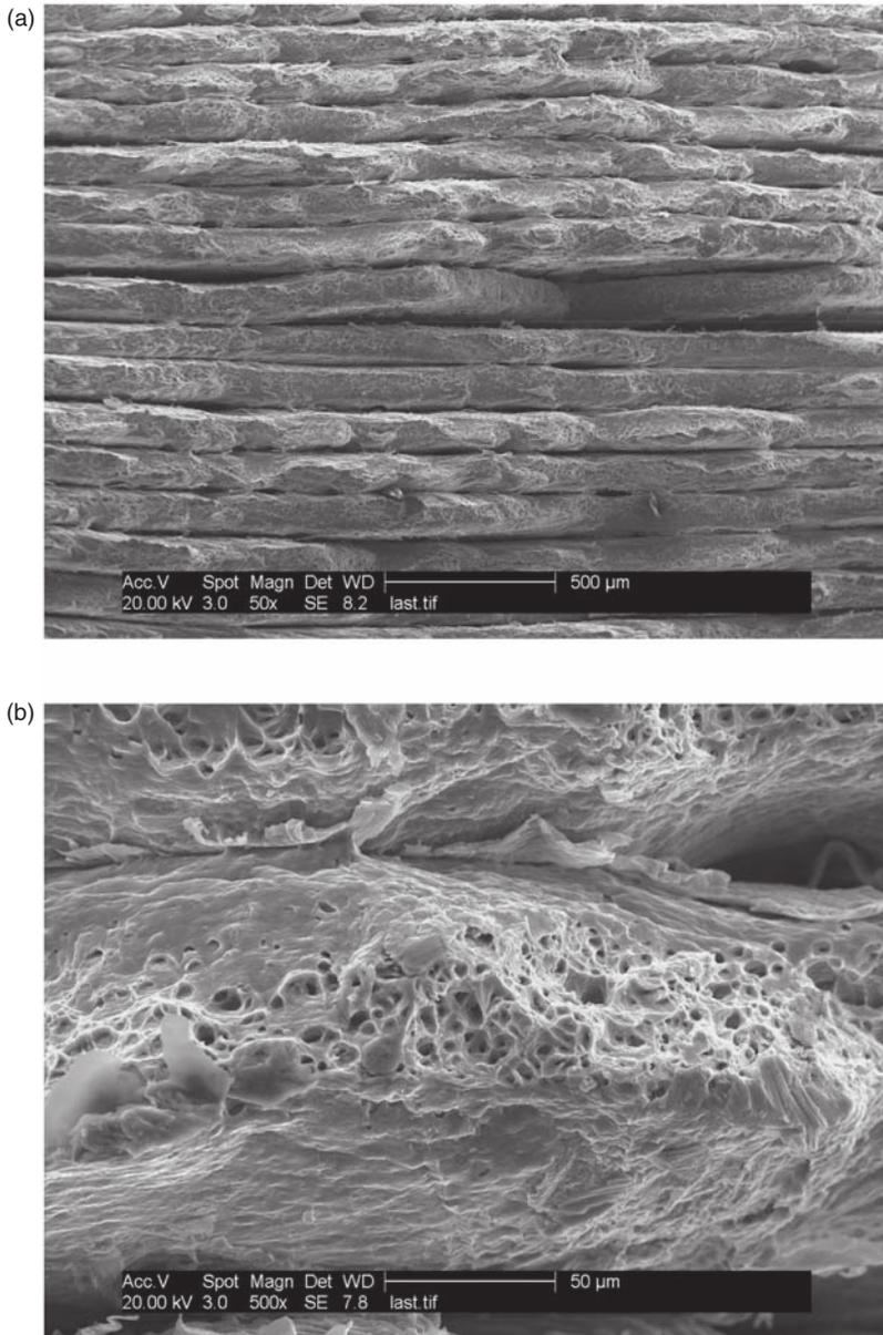
**Figure 11.** Tensile fracture surface of a Type I specimen: (a) low magnification and (b) high magnification.
