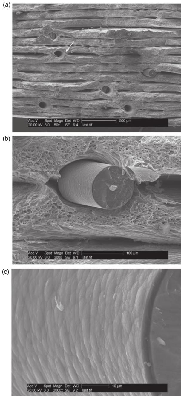
**Figure 12.** Tensile fracture surface of a Type II specimen: (a) low magnification (arrow indicates enhanced bonding in the vicinity of the fiber), (b) high magnification, and (c) exterior surface of a SiC fiber at high magnification.
