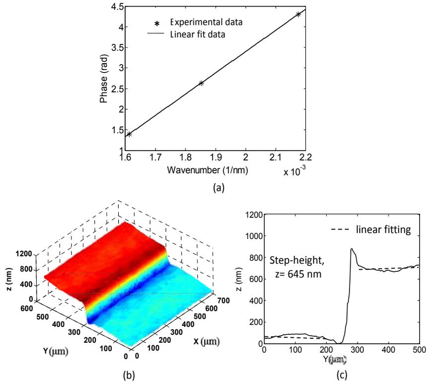
Fig. 4. Surface profile analysis using the fringe order method: (a) The linear fitting of the adjusted phase values measured at three wavelengths at a given pixel, (b)  $2\pi$  ambiguity corrected single wavelength 3-D surface profile of an etched silicon sample using the phase at  $\lambda_1$ , and (c) line scan profile showing the step height 645 nm.
