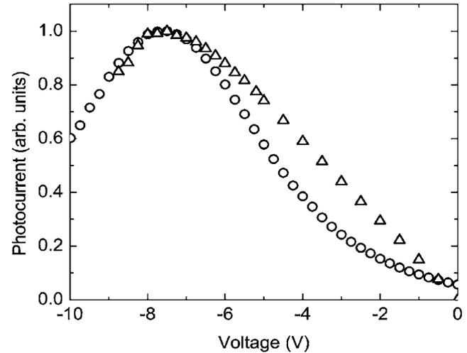
FIG. 8. A plot of the measured (○) and calculated [Δ, by using Eq. (5)] photocurrents as a function of applied reverse bias.
