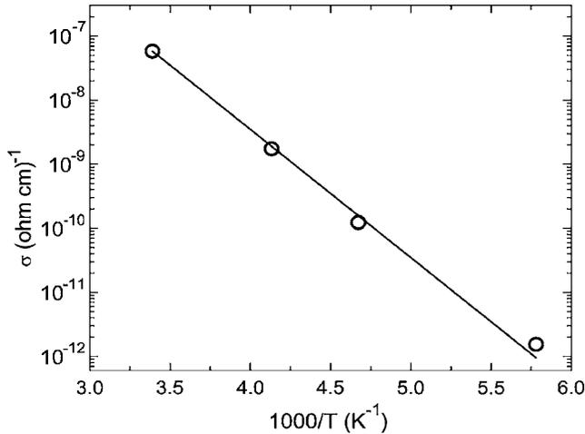
FIG. 1. A plot of conductivity as a function of  $1000/T$  for a planar doped TPD sample. The activation energy of the conductivity is 0.38 eV.
