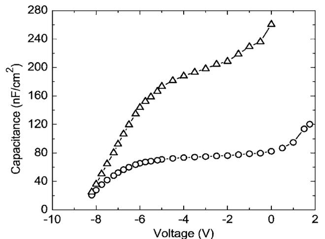
FIG. 5. A plot of the voltage dependence of the capacitance for a 2000 Å thick TPD device. The plot shows the measured capacitance ( $-O-$ ) and  $C_{ins}$  ( $-\Delta-$ ).  $C_{ins}$  was calculated by assuming that the capacitance at slight forward bias is the measure of  $C_{sc}$ .
