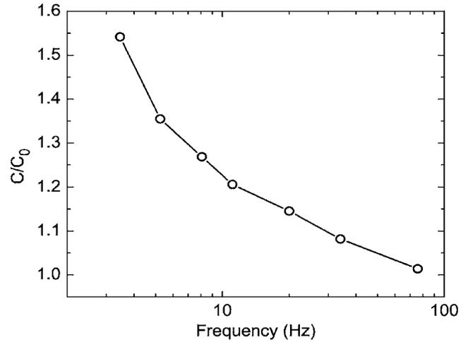
FIG. 4. A plot of the frequency dependence of the capacitance ( $C_0$  is the geometric capacitance) for a F<sub>4</sub>-TCNQ doped AlQ<sub>3</sub> sample.
