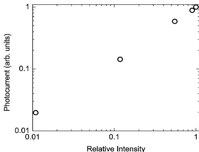
FIG. 9. A plot of the intensity dependence of the photocurrent for a planar TPD device.
