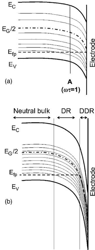
FIG. 3. The energy level alignment of a doped TPD device near the Al electrode is shown (a) when the device is at small reverse bias and (b) when it is at large reverse bias. DR and DDR are acronyms for the depletion region and deep depletion region, respectively.
