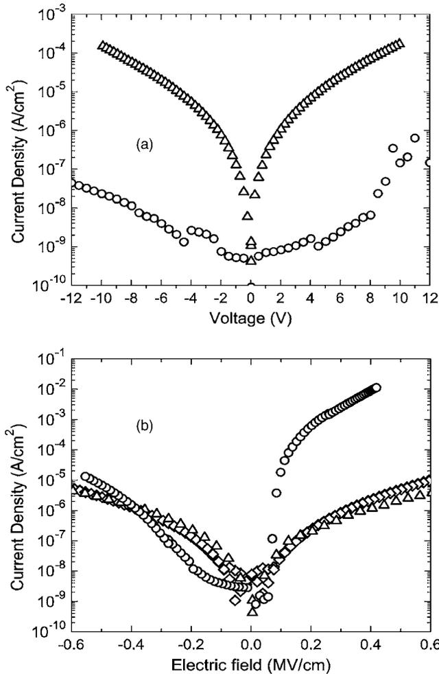
FIG. 7. The dark current voltage plot of a neat polycarbonate film (○) and one where  $F_4$ -TCNQ is added to it (Δ) are shown in graph (a). Graph (b) compares the dark current for  $F_4$ -TCNQ doped TPD (○),  $AlQ_3$  (◇), and polycarbonate (Δ) films.
