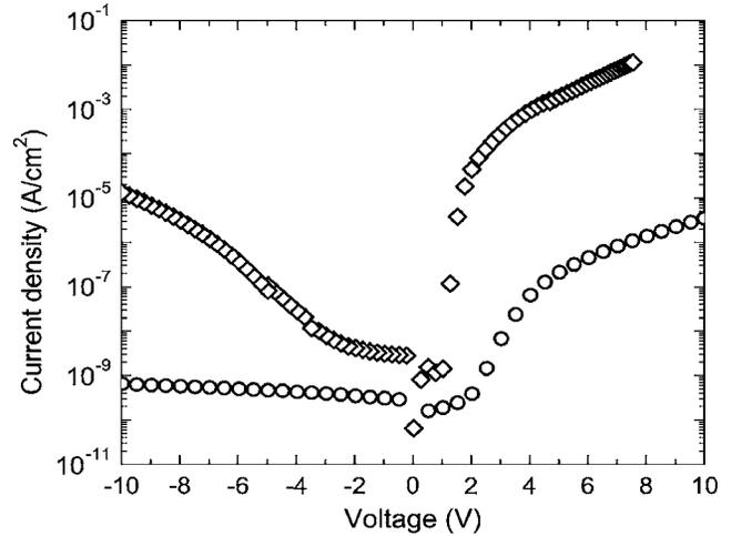
FIG. 6. A plot of the dark current density as a function of voltage for 2000 Å thick samples of (a) undoped TPD (○) and (b) doped TPD (◇).
