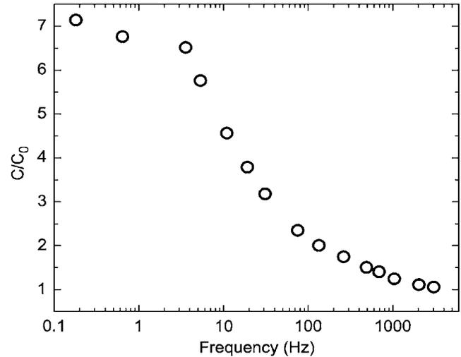
FIG. 2. A plot of the frequency dependence of the normalized capacitance  $C/C_0$  ( $C_0$  being the geometrical capacitance) for a doped TPD sample. For frequency less than 5 Hz, the capacitance was recorded by measuring the displacement current. The value of  $C_0$  is 14 nF/cm<sup>2</sup>.
