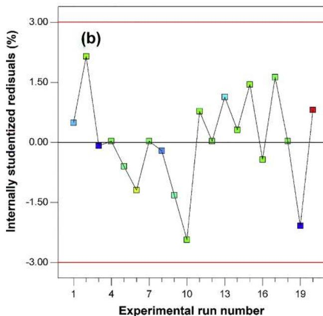
Fig. 8. (a) COD removals observed in experiments and predicted by RSM, and (b) the COD residuals obtained in CCD experiment.
