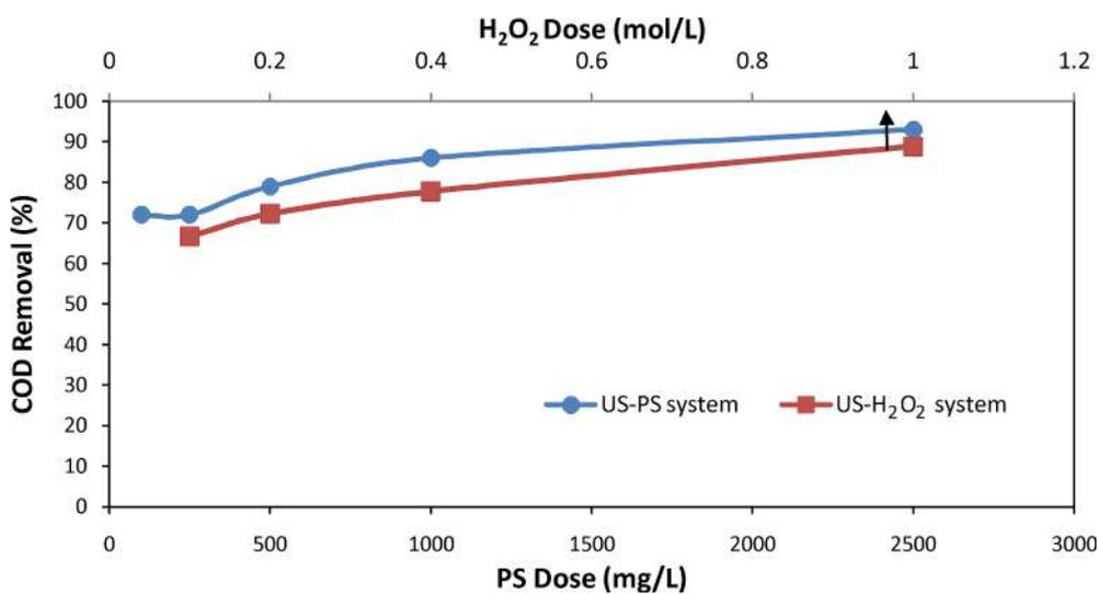
Fig. 6. Effect of PS and H<sub>2</sub>O<sub>2</sub> dosages on COD removal at 30% US amplitude and 10 min US irradiation.
