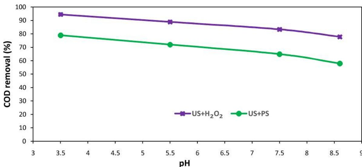
Fig. 7. Effect of pH on COD removal in US-PS (1000 mg/L) and US-H<sub>2</sub>O<sub>2</sub> (1 mol/L) system (10 min at 30% US amplitude).
