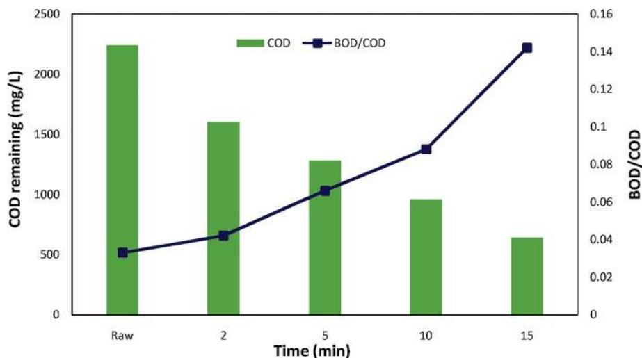
Fig. 4. Effect of irradiation time on COD remaining and BOD/COD ratio in US-alone system at 30% US amplitude.
