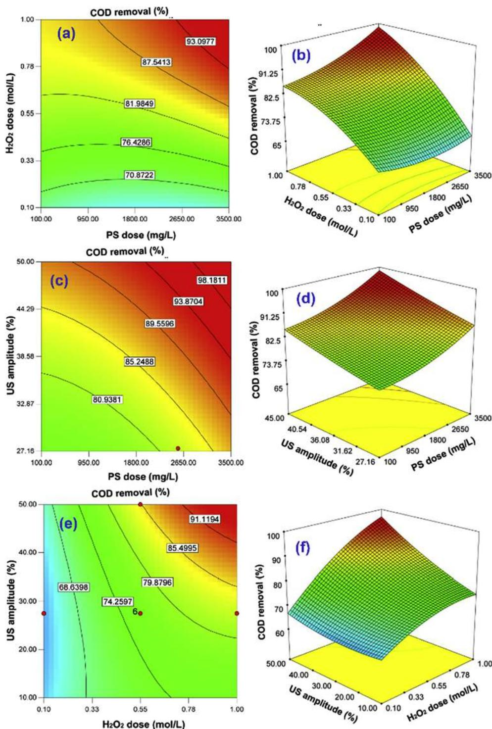
Fig. 9. Contour and response surface plots showing the effect of PS dose, H<sub>2</sub>O<sub>2</sub> dose and US amplitude on COD removal (%).
