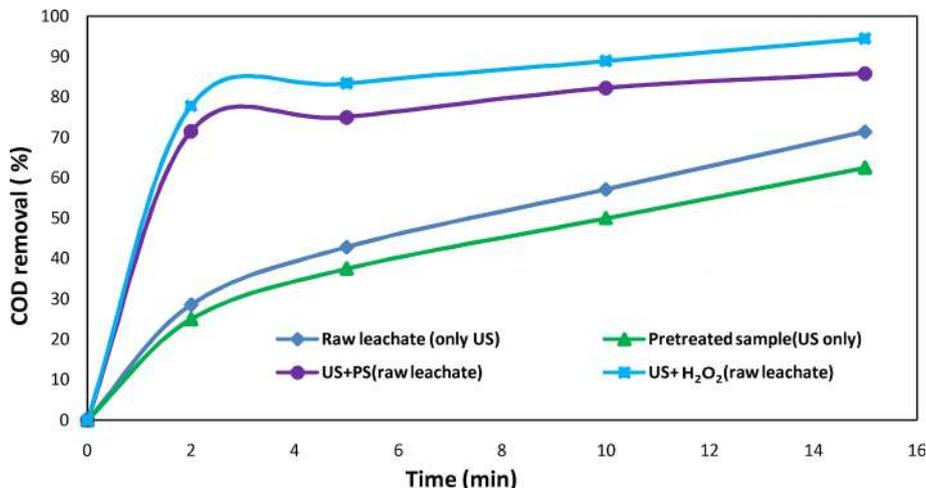
Fig. 2. Comparison of COD removal efficiency in different US systems at 30% amplitude.
