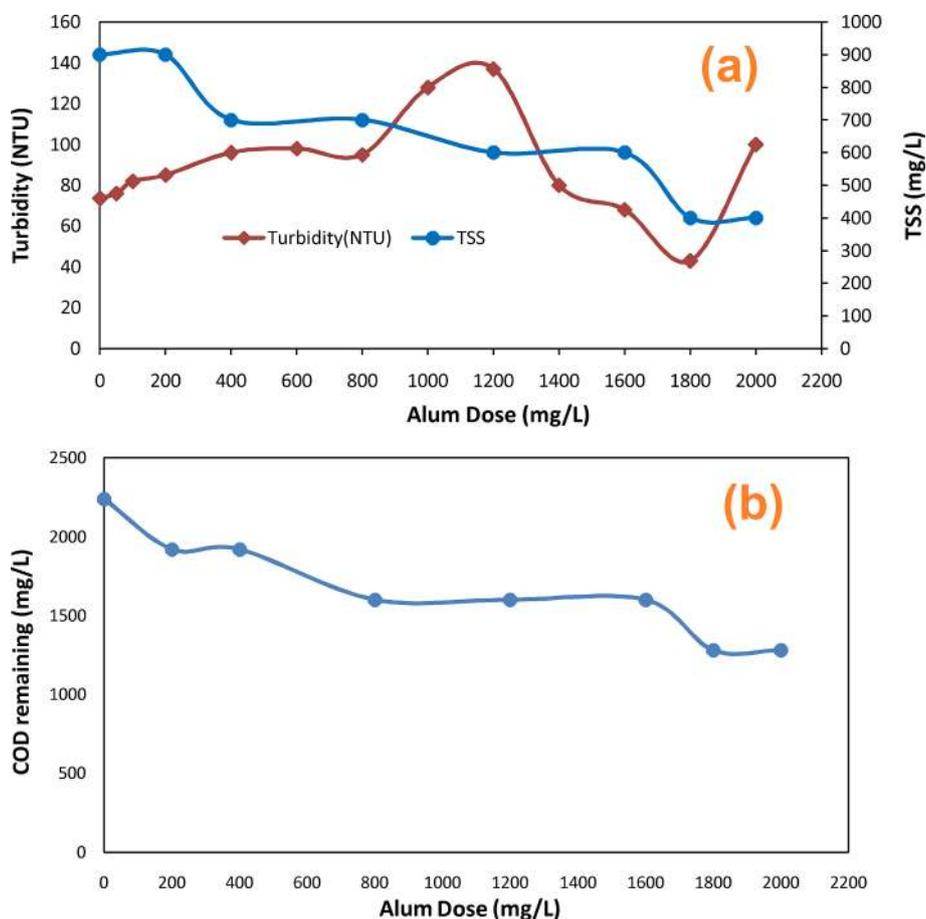
Fig. 1. Effect of coagulant dose on a) turbidity and TSS removal and b) COD removal from landfill leachate.
