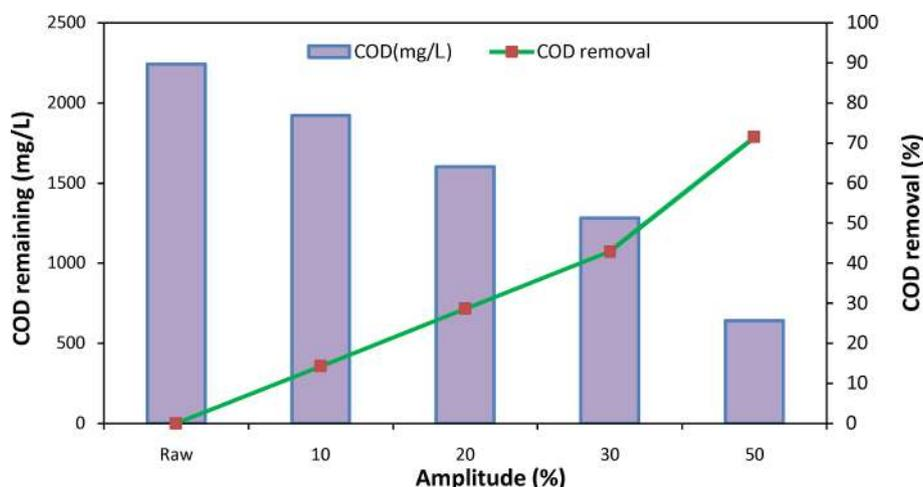
Fig. 3. Effect of US-amplitude on COD removal in US alone system after a reaction time of 5 min.
