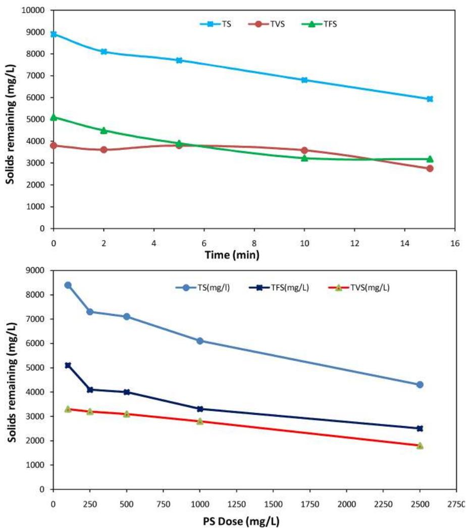
Fig. 5. Solids remaining at 30% US amplitude with respect to a) US irradiation time in US-alone system, and b) PS dosage in US-PS system after 10 min.
