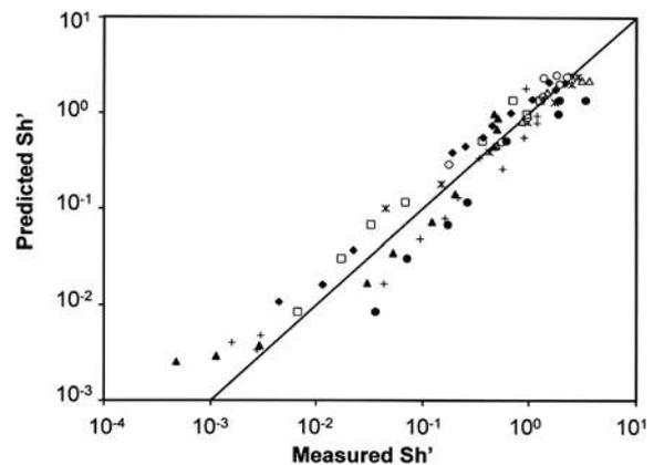
**Figure 3.** Predicted Sherwood numbers estimated from the new local mass transfer correlation (equation (6)) versus observed Sherwood numbers calculated from experimental concentration data. Each set of symbols represent data from one of seven different experiments.
