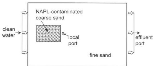
**Figure 1.** Front view of the two-dimensional cell experimental cell used by *Nambi and Powers* [2000]. Dimensions of the cell are 17.8 cm × 12 cm × 2.9 cm. The size and number of coarse sand lenses, initial NAPL saturation within the coarse sand lens, and ratio of permeability in the fine to coarse sand were varied between experiments. Mechanisms within the coarse sand lens that affect NAPL dissolution rates were the focus of this first paper.
